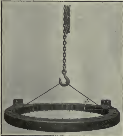
30 DEGREE ANGLE SLING, WRONG WAY.
