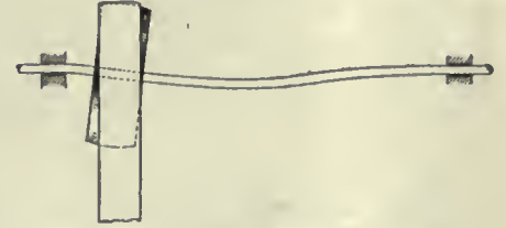
FIG. 2. EXAGGERATED EFFECT OF A TIGHT BELT.
