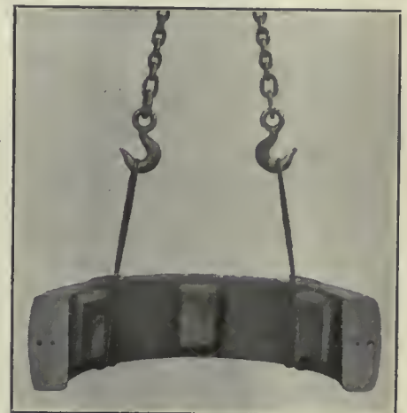
PROPER METHOD OF MAKING HITCH. THE FRICTION OF CABLE AROUND THE OBJECT GIVES APPROXIMATELY A TWO PART CABLE.
