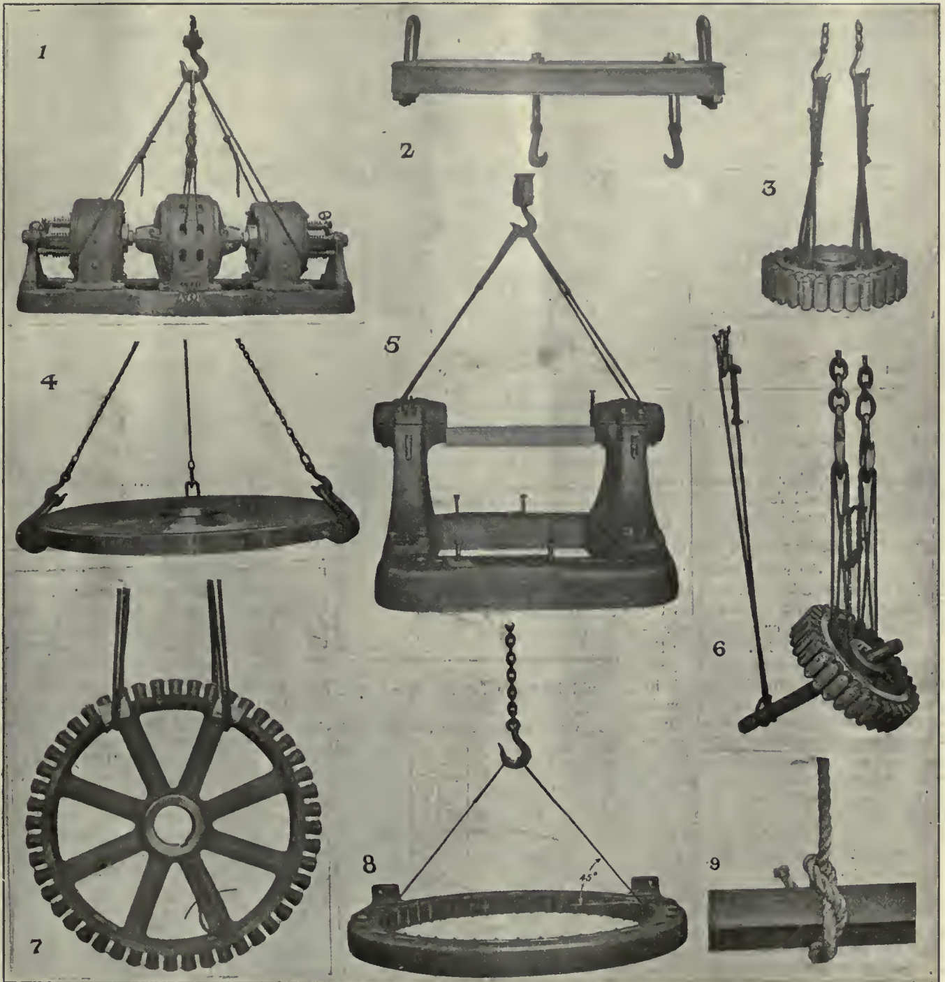
FIG. 1. PROPER WAY OF LIFTING THREE UNIT SET. FIG. 2. EQUALIZER USED WITH TWO CRANES. FIG. 3. METHOD OF LIFTING AND TURNING REVOLVING FIELDS, FIRST POSITION. FIG. 4. RIGHT WAY OF LIFTING PLATE WITH THREE HOOKS. FIG. 5. METHOD OF LIFTING BASE AND STANDARDS. FIG. 6. METHOD OF LIFTING AND TURNING REVOLVING FIELDS, SECOND POSITION. FIG. 7. RIGHT WAY TO LIFT REVOLVING FIELD. FIG. 8. 45 DEGREE ANGLE SLING, RIGHT WAY. FIG. 9. TIMBER HITCH.
