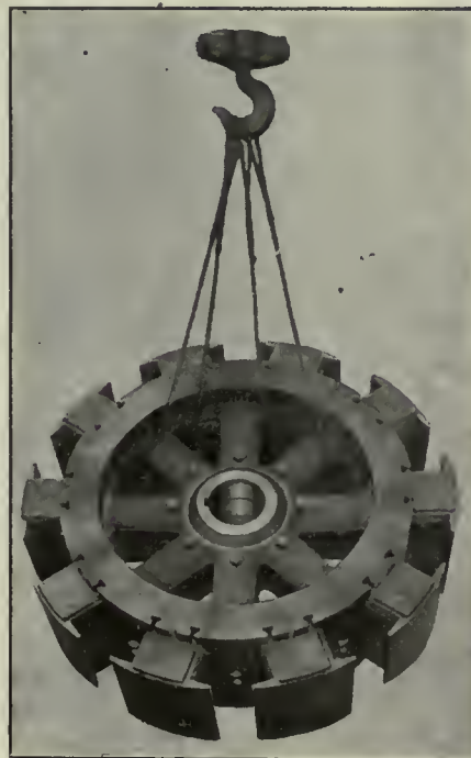
PROPER METHOD OF MAKING HITCH FOR TURNING REVOLVING FIELD, STRAIN BEING EQUALIZED.
