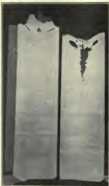
FIGS. 5, 6. SECTIONS OF COMPRESSED AND UNCOMPRESSED STEEL INGOTS.
