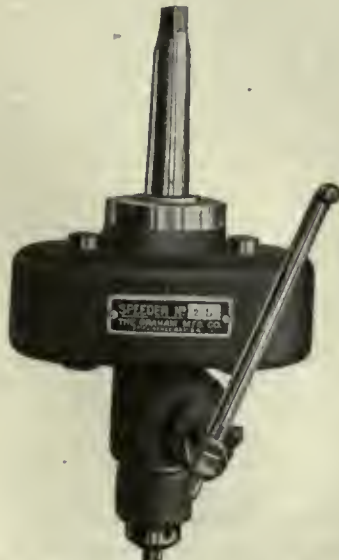
FIG. 6. SHOWING STYLE HAVING SENSITIVE FEED LEVER.
