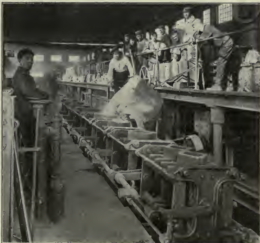
FIG. 4. CASTING THE INGOTS FROM AN HYDRAULICALLY OPERATED TOP POUR LADLE.
