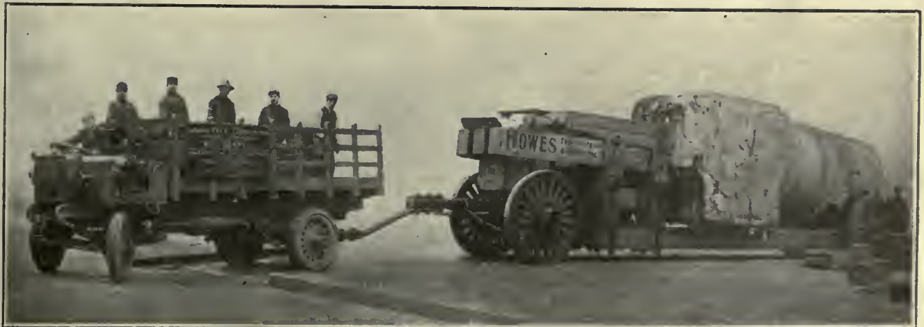
VIEW OF THE LA FRANCE TRUCK WITH ITS OWN LOAD AND THE TRAILING LOAD.
