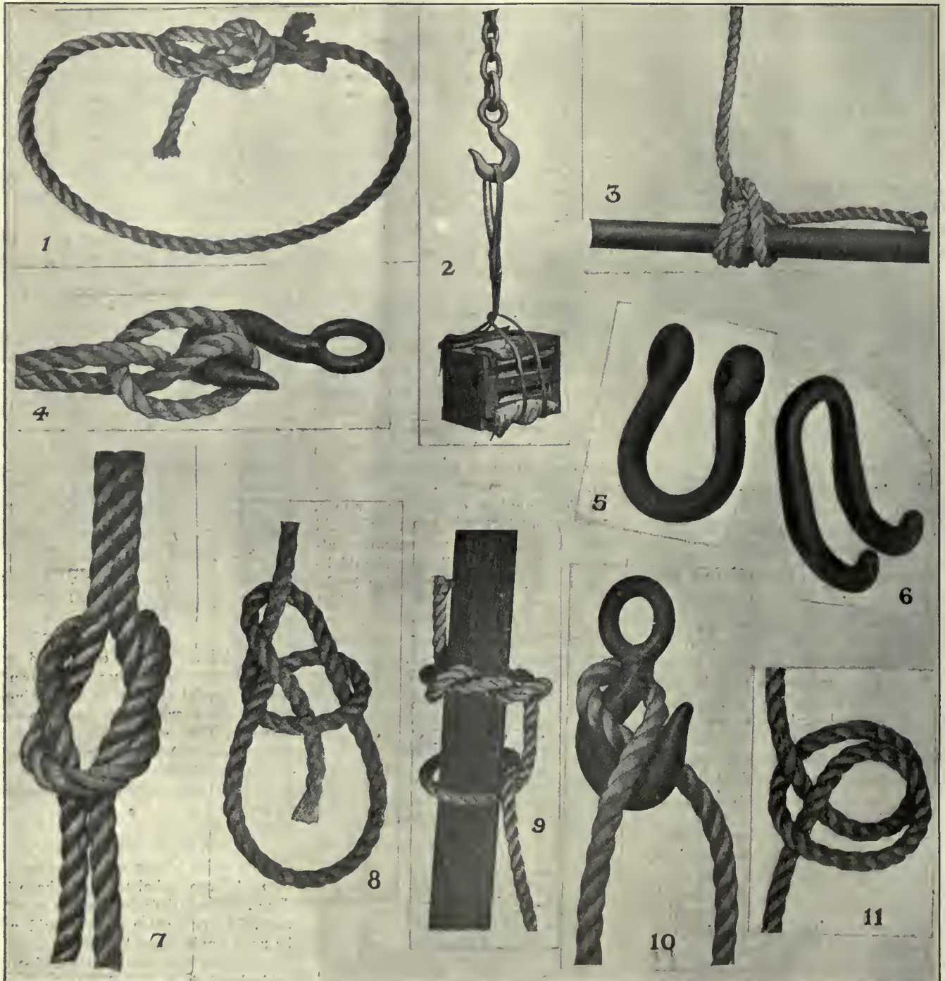
FIG. 1. SHEET BEND IN EYE. FIG. 2. DOUBLE CABLE SLING, RIGHT WAY TO LIFT LOAD. FIG. 3. STUDDING SAIL HITCH. FIG. 4. CLOVE OR DOUBLE HALF HITCH. FIG. 5. SHACKLE. FIG. 6. DOUBLE HOOK. FIG. 7. SQUARE OR REEF KNOT. FIG. 8. BOWLINE COMPLETE. FIG. 9. TIMBER HITCH AND HALF HITCH. FIG. 10. BLACKWALL HITCH. FIG. 11. CLOVE OR DOUBLE HALF HITCH.
