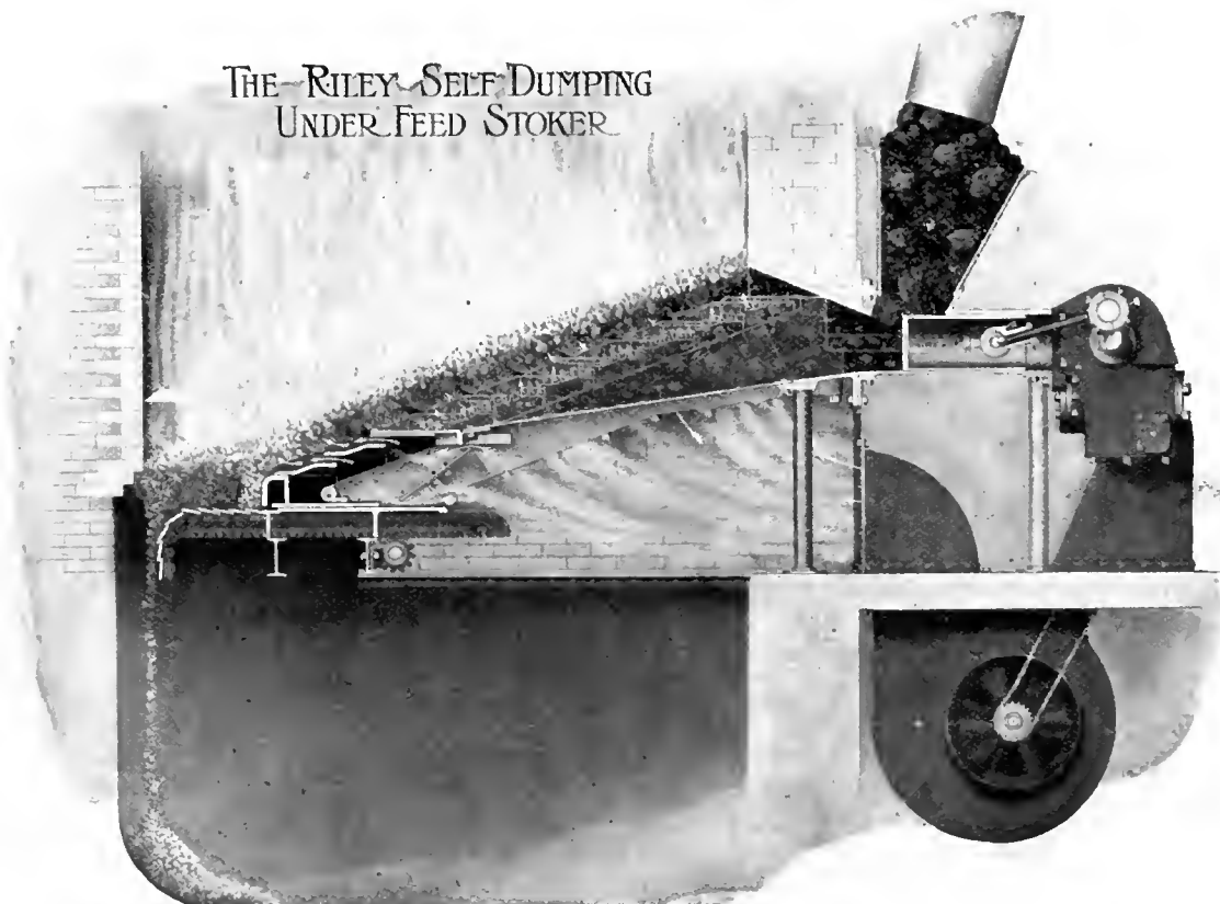
FIG. 1. SECTIONAL VIEW THROUGH STOKER.
