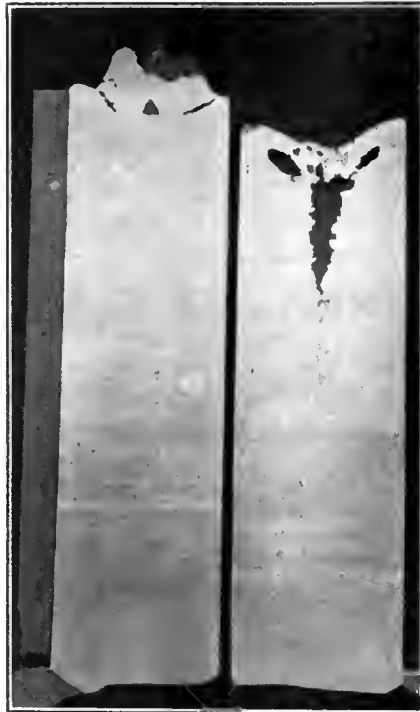
FIGS. 5, 6. SECTIONS OF COMPRESSED AND UNCOMPRESSED STEEL INGOTS.
