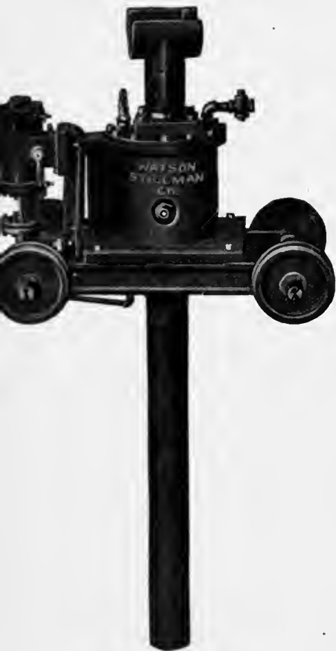
IMPROVEMENT IN HYDRAULIC PIT JACKS.
