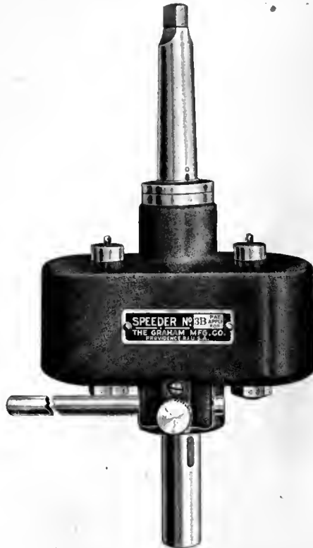
FIG. 5. SHOWING SPINDLE FOR TAPER SHANK DRILLS INSTEAD OF CHUCK.
