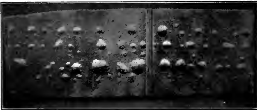
PHOTOGRAPH OF BLISTERED STEEL SHEET.
