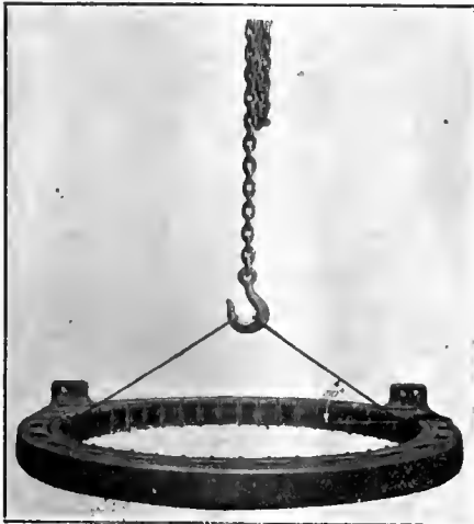
30 DEGREE ANGLE SLING, WRONG WAY.
