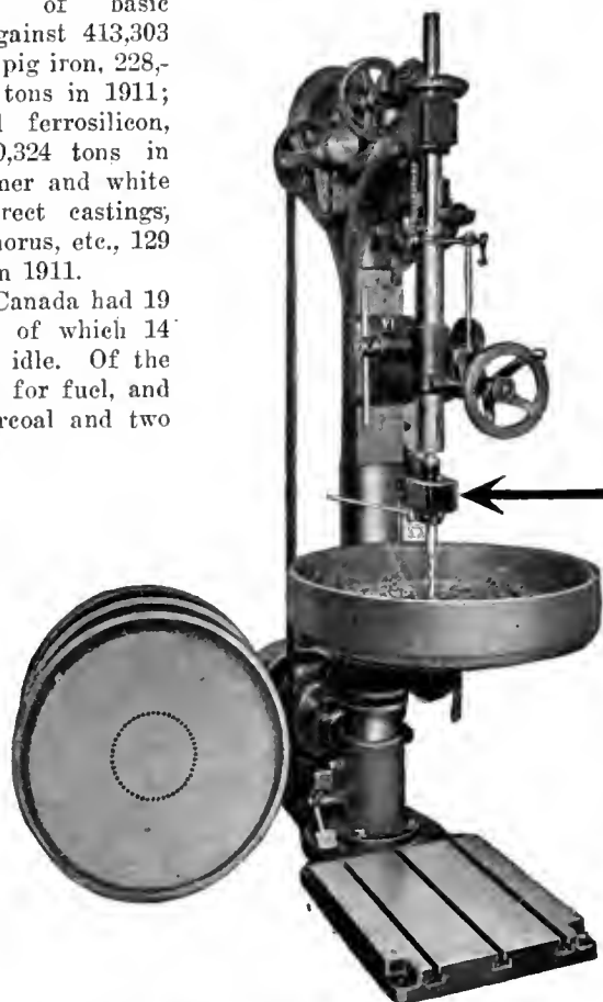
FIG. 8. EXAMPLE OF DRILLING 7-16 IN. HOLES IN BOILER HEADS 11-16 IN. THICK.
