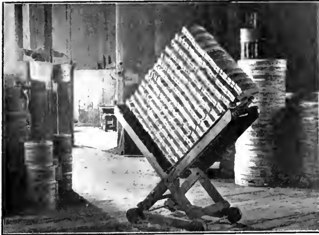
FIG. 5. SEGMENTS READY FOR FORMING INTO RINGS. ILLUSTRATION SHOWS CONVENIENT TRUCK BY WHICH THEY ARE MOVED ABOUT THE SHOP.
