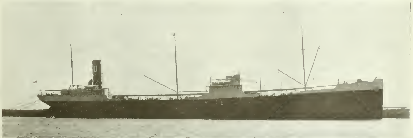
STEAMSHIP "LA BREA," PROPELLED BY 2,600 HORSE POWER "CURTIS" TURBINE DRIVING THROUGH "ALQUIST" REDUCTION GEARS.
