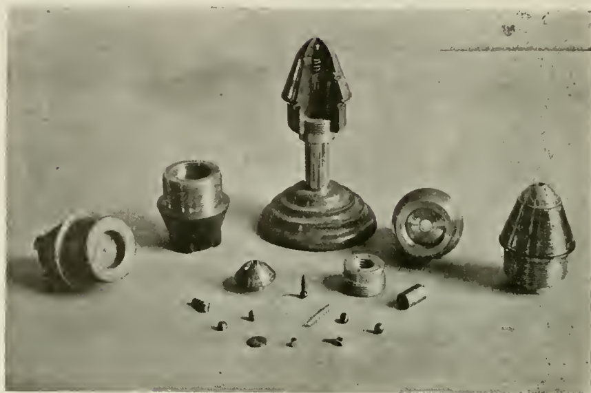
FIG. 13. VIEWS OF FUSE AND ITS COMPONENT PARTS.
