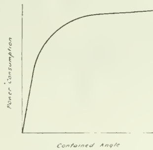
FIG. 5. PROBABLE RELATION BETWEEN CONTAINED ANGLE OF CUTTING TOOL AND POWER.
