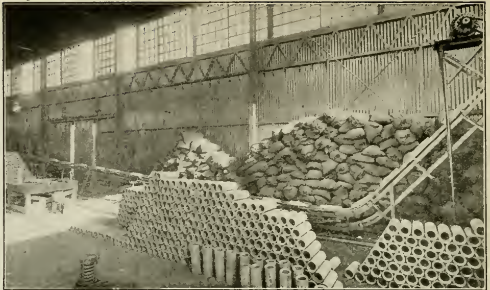
FIG. 3—SHELL FORGINGS BEING CONVEYED FOR LOADING ON CARS.
