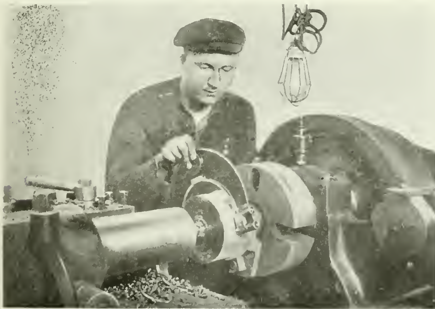
FIG. 10. SIZING ADAPTERS PREPARATORY TO THREADING.
