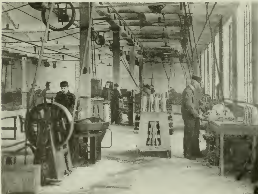
FIG. 12. BANDING DEPARTMENT, SHOWING HYDRAULIC PRESS WITH "ROELOFSON" BAND TURNING MACHINE AT RIGHT.
