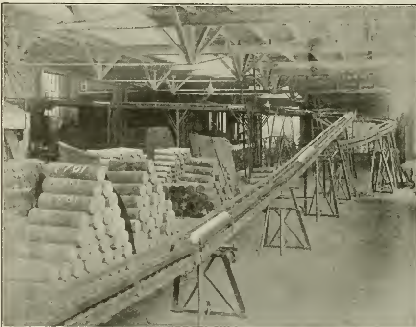
FIG. 2—PORTION OF CONVEYOR TRANSFERRING BILLETS DIRECT FROM CARS TO BATTERY OF CONTINUOUS FURNACES.
