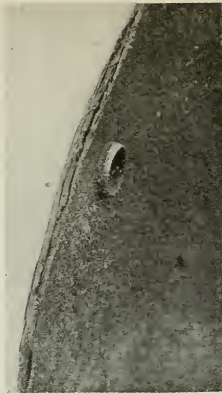
LAMINATIONS IN EDGE OF FRACTURED COVER.
