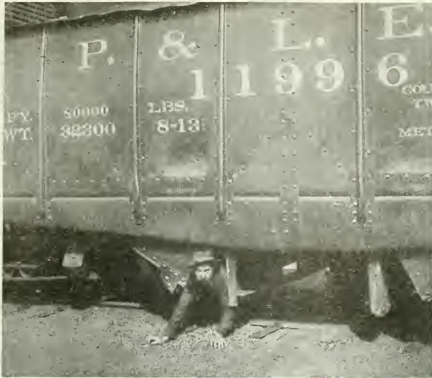
FIG. 24. UNSAFE PRACTICE; CRAWLING OUT OF HOPPER CAR THROUGH HOPPER OPENING.
