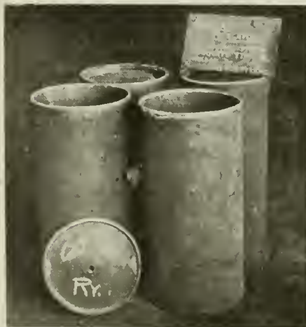
GROUP OF CYLINDERS RECLAIMED BY OXY-ACETYLENE WELDING
