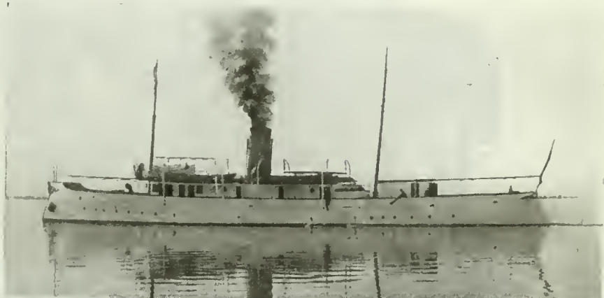
CANADIAN GOVERNMENT FISHERIES PATROL BOAT "VIGILANT," 176 FT. x 22 FT. x 14 FT. 3 INS., BUILT BY POLSON IRON WORKS.
