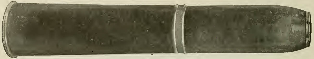
BRASS CARTRIDGE CASE WITH 18-PDR. SHRAPNEL SHELL INSERTED.
