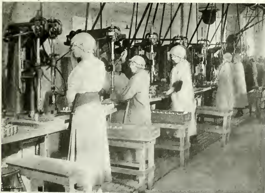
FIG. 5. BATTERY OF "HENRY & WRIGHT" DRILLS ON BODY DETAIL OPERATIONS.
