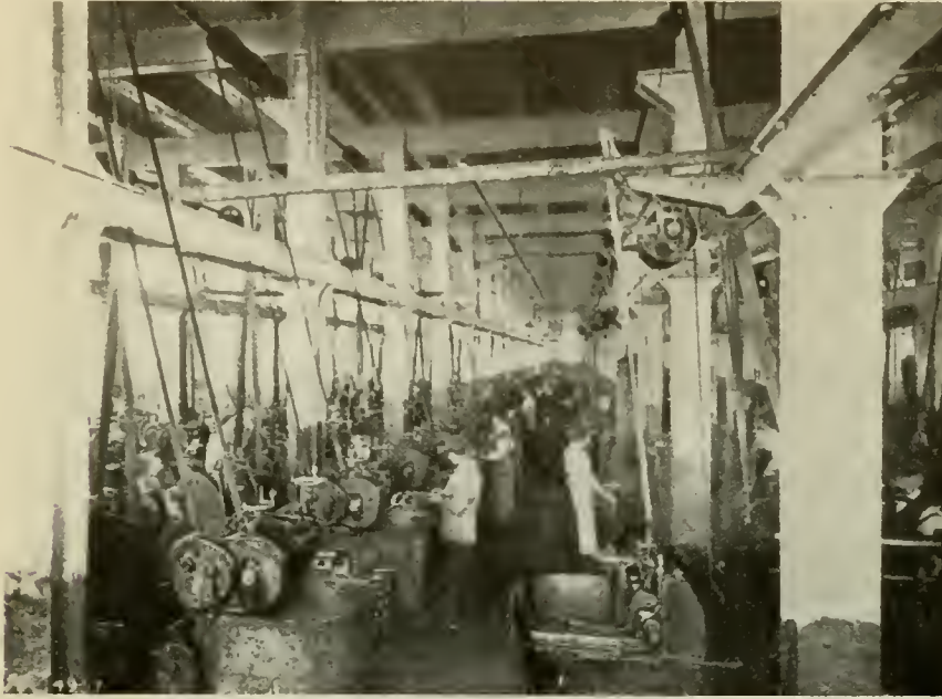
BLOCK OF 120 AUTOMATIC MILLING MACHINES.
