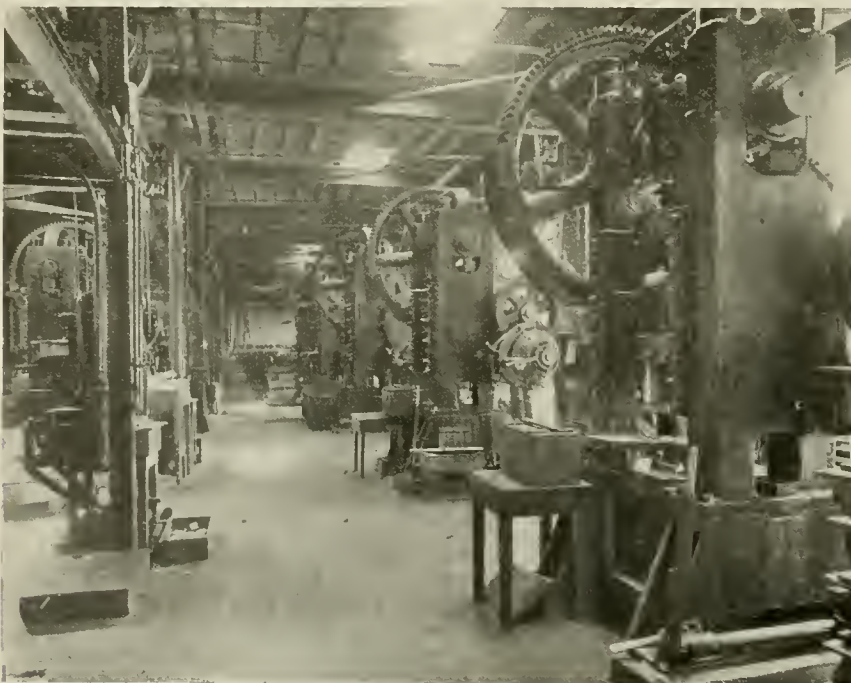
HEAVY DRAW PASSES FOR EARLIER DRAWING OPERATIONS.
