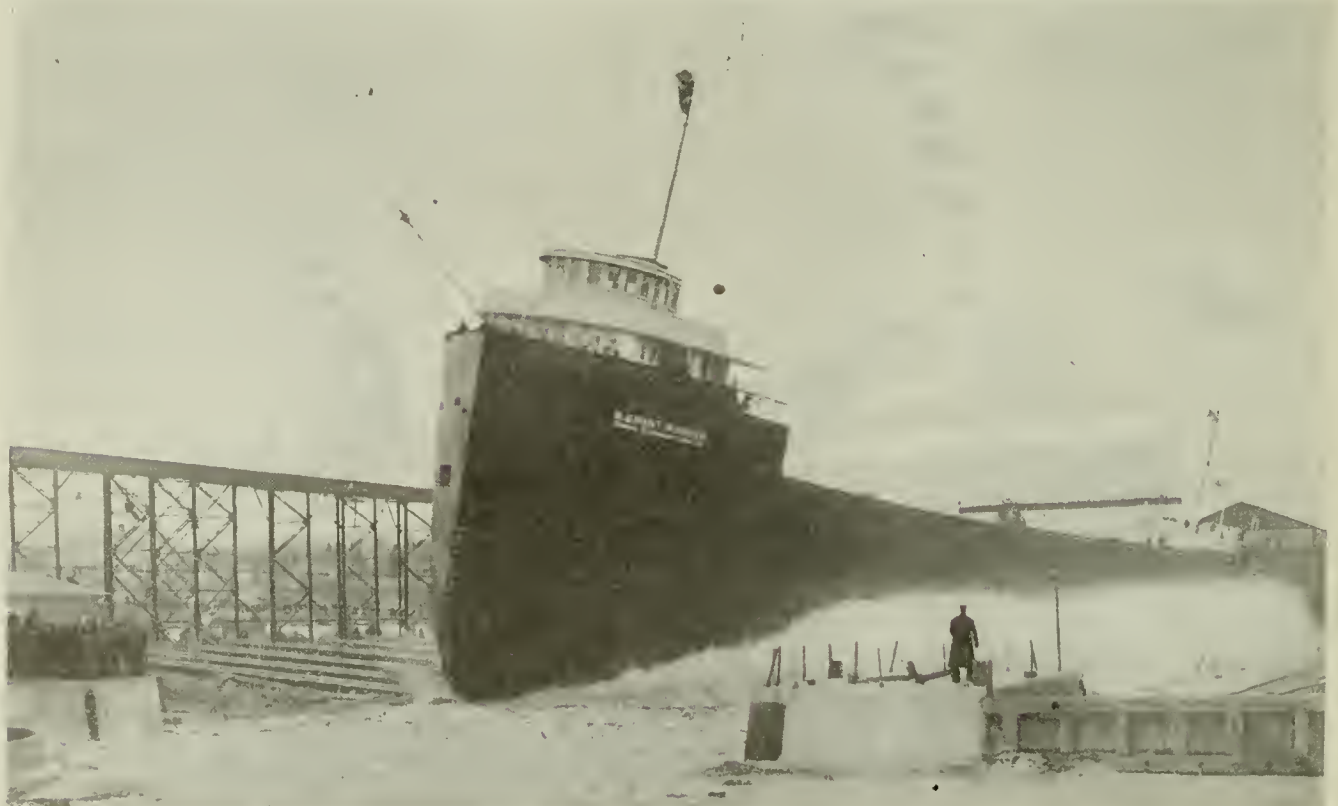
625-FT. FREIGHTER "W. GRANT MORDEN" BEING LAUNCHED FROM THE YARD OF THE WESTERN DRYDOCK & SHIPBUILDING CO., PORT ARTHUR, ONT.
