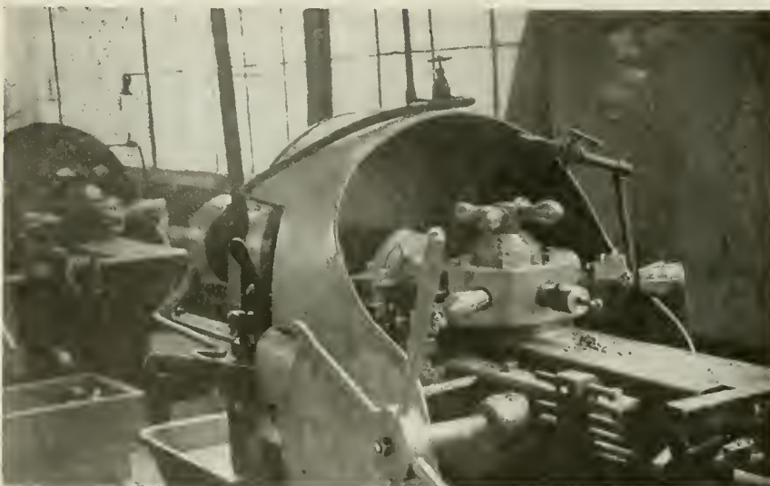
FIG. 2. STECHER TURRETS FINISHING FUSE BODIES.
