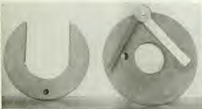
FIG. 1. VIEWS OF ECCENTRIC AND EXTERIOR OF FIRST GOVERNOR WITH SINGLE CRANK ARM.
