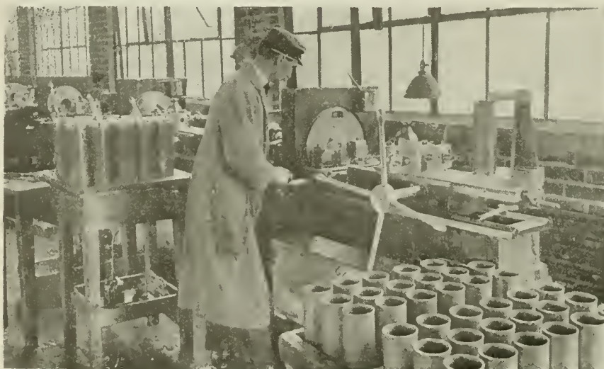
MACHINING HEADS OF CARTRIDGE CASES ON "BULLARD" TURRET LATHE. THE CASE MOUTHS ARE TRIMMED ON THE SAME MACHINES.
