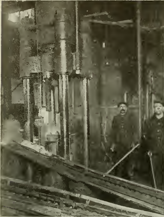
500-TON, 6-INCH SHELL FORGING PRESS WITH GRAVITY CARRIER IN FRONT.
