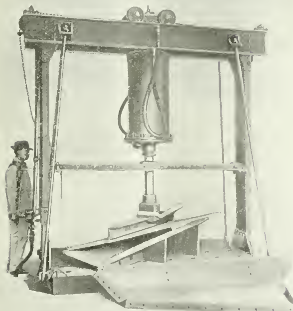
RECLAIMING PRESS FORMING HOPPER SHEETS FOR STEEL CARS.
