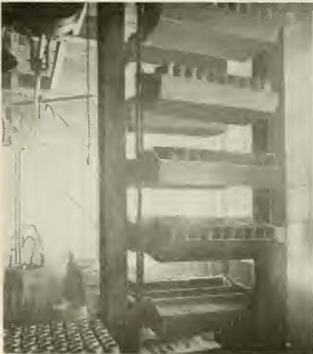
FIG. 11. SPECIAL CONVEYOR IN CONNECTION WITH SHELL NOSE ANNEALING OPERATION.
