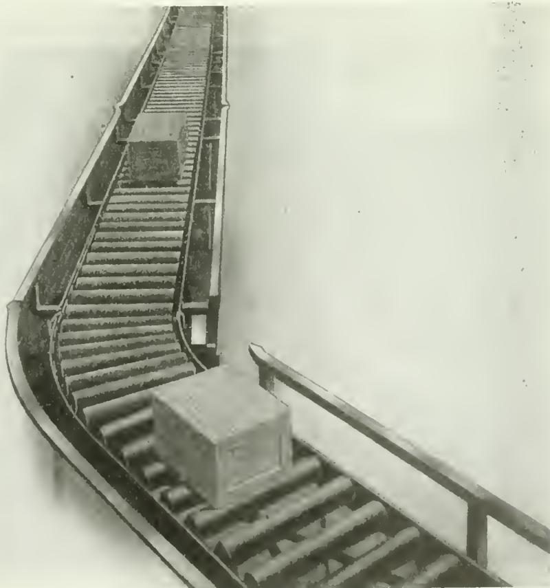
FIG. 1. STEEL BALL-BEARING GRAVITY ROLLER BOX CARRIER OF 1% GRADE.
