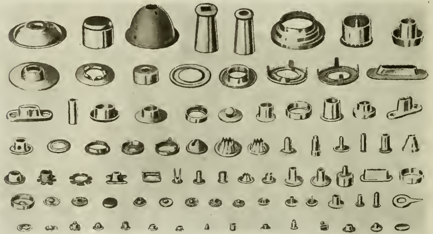
SPECIMENS OF WORK PRODUCED ON MULTIPLE PLUNGER PRESS.
