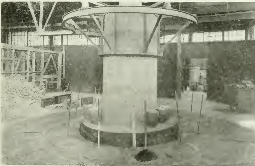
TWELVE CRUCIBLE CAPACITY FURNACE FOR MELTING BRASS SCRAP FROM CARTRIDGE CASES.
