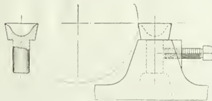
FIG. 6. AUTHOR'S SMALL ANGLE TOOL AND FIG. 7. TOOL HOLDER.
