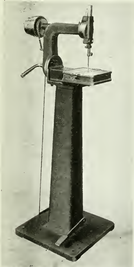
FILING MACHINE WITH OVERHUNG SWIVELING HEAD AND ADJUSTABLE FILE SUPPORT.
