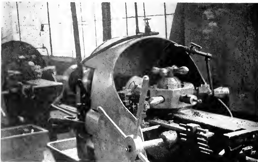
FIG. 2. STECHER TURRETS FINISHING FUSE BODIES.
