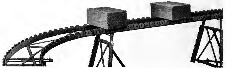
FIG. 3. STEEL BALL-BEARING GRAVITY WHEEL BOX CARRIERS OF 4% GRADE.
