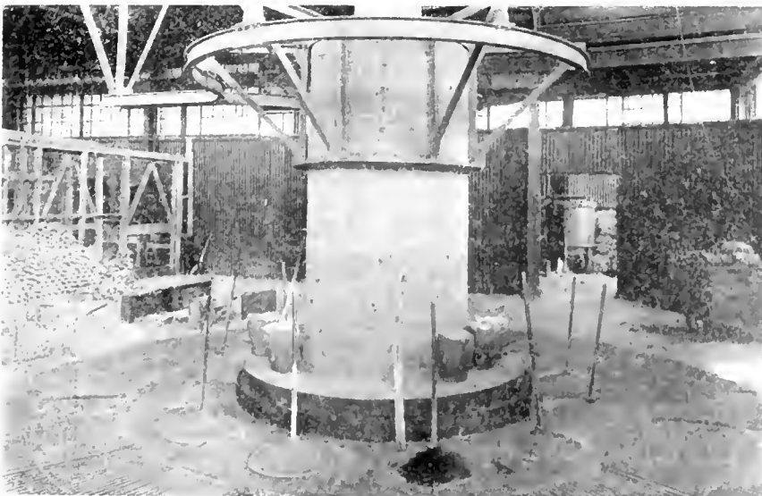
TWELVE CRUCIBLE CAPACITY FURNACE FOR MELTING BRASS SCRAP FROM CARTRIDGE CASES.
