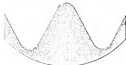
FIG. 7. COMARISON OF THE PROJECTED IMAGE AND TRUE SCREW THREAD OUTLINE
