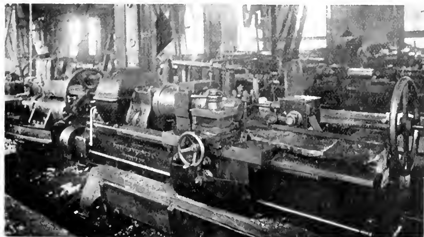
WAVING AND GROOVING ON BAWDEN LATHE EQUIPPED WITH VICTORIA FOUNDRY CO. ATTACHMENT.
