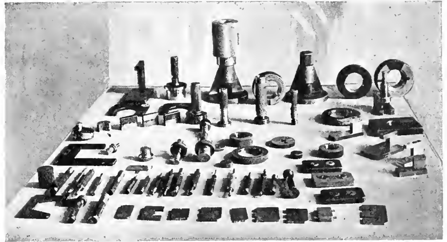
FIG. 15. SOME OF THE GAUGES USED TO SECURE ACCURACY IN PRODUCTION.
