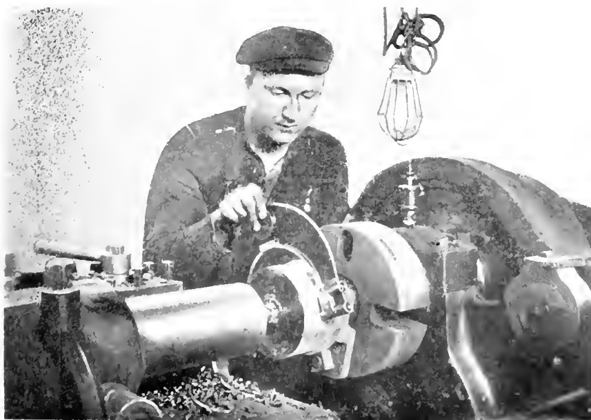
FIG. 10. SIZING ADAPTERS PREPARATORY TO THREADING
