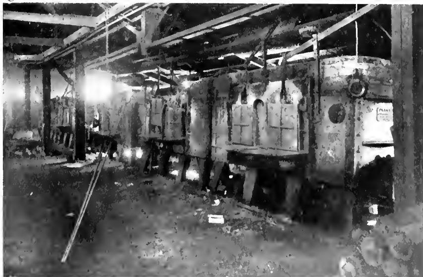
ROW OF BATCH FURNACES SHOWING SUSPENDED TONGS USED FOR HANDLING BILLETS.
