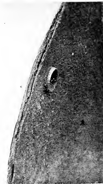
LAMINATIONS IN EDGE OF FRACTURED COVER.
