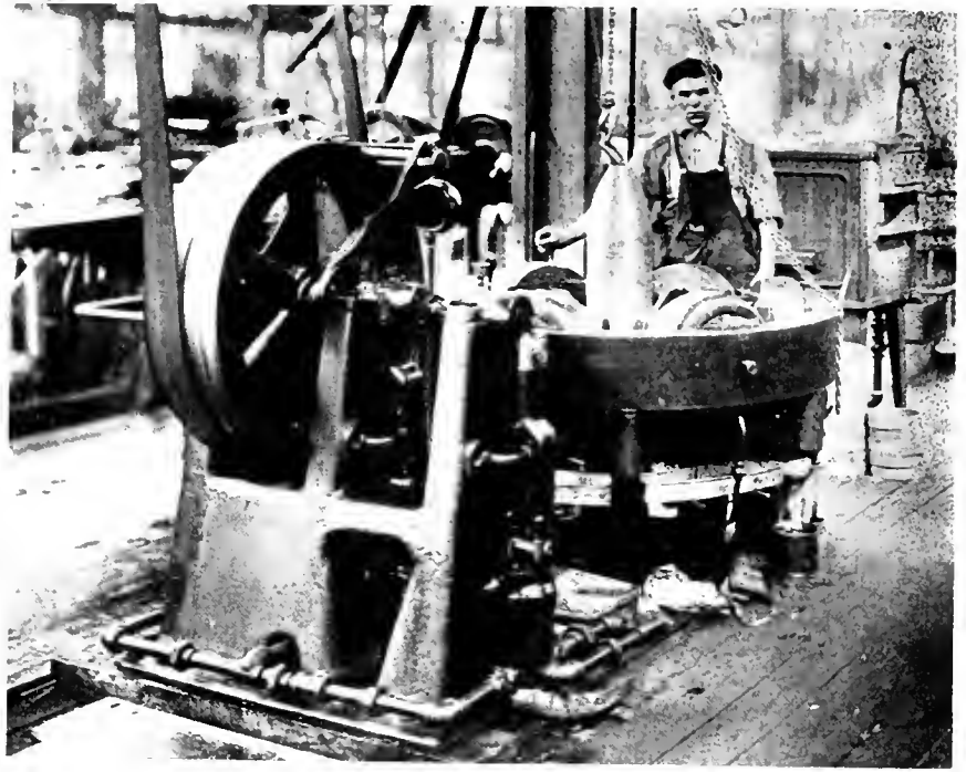
FIG. 13. COPPER BANDING EQUIPMENT.
