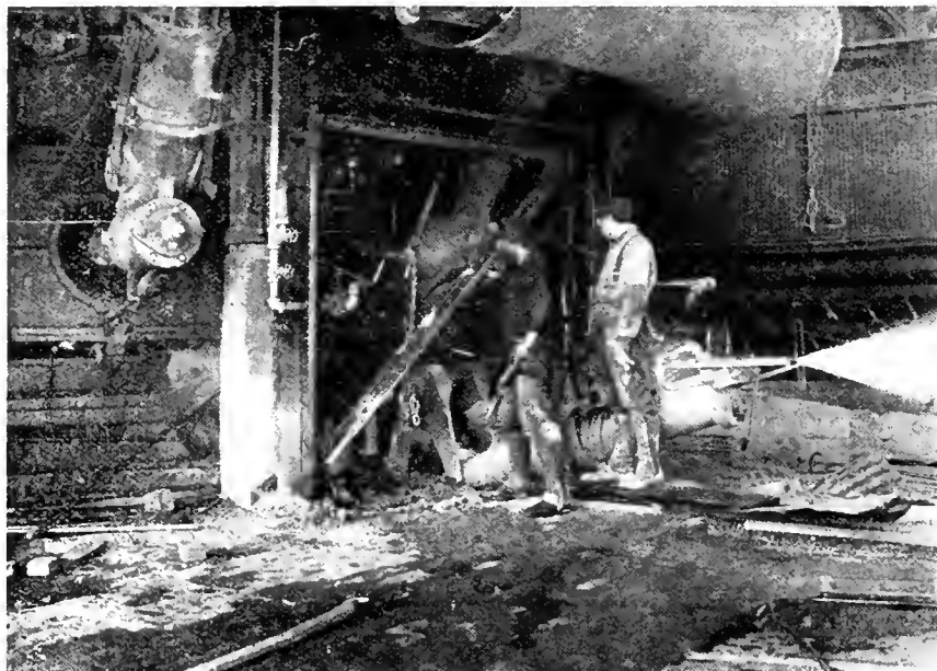
FIG. 18. SAFE WAY TO STOP TAPPING HOLE. Helper is using shovel and standing away from the trough and the tapping hole.
