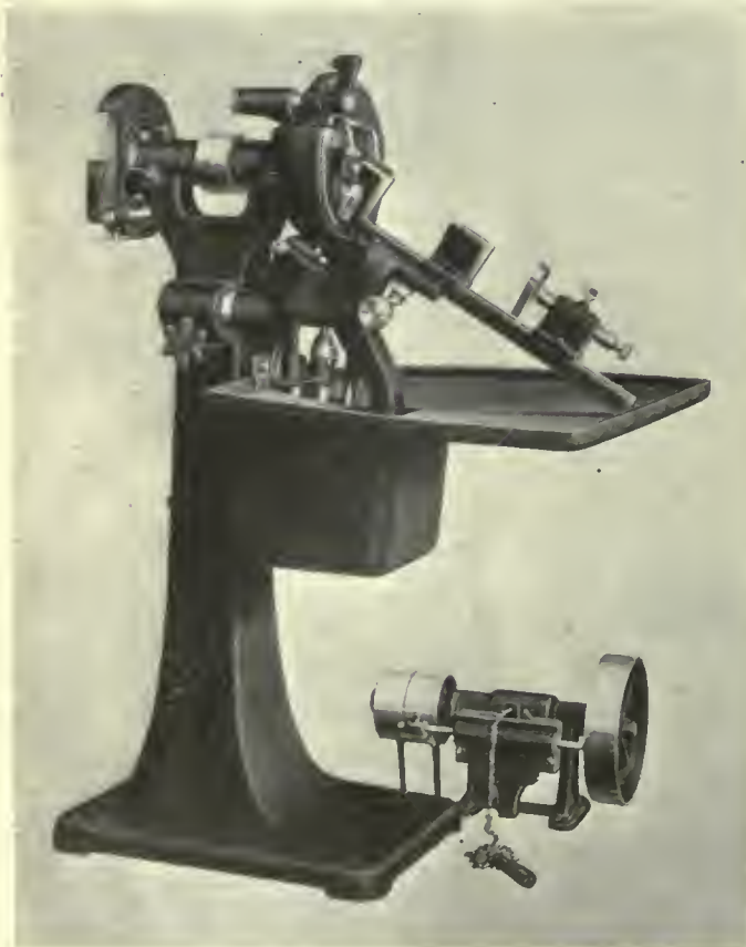
DRILL GRINDER WITH PAN AND COOLANT RESERVOIR
