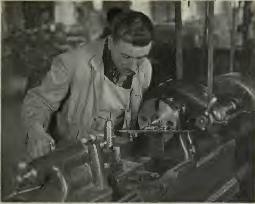
SETTING THE COMPOUND REST
