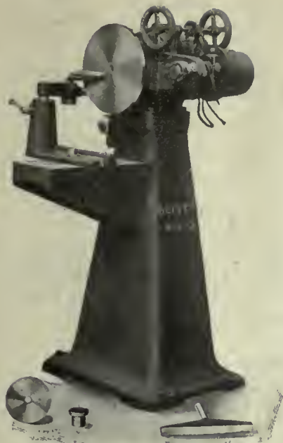
REAR VIEW OF ALTERNATING CURRENT FACE LATHE
