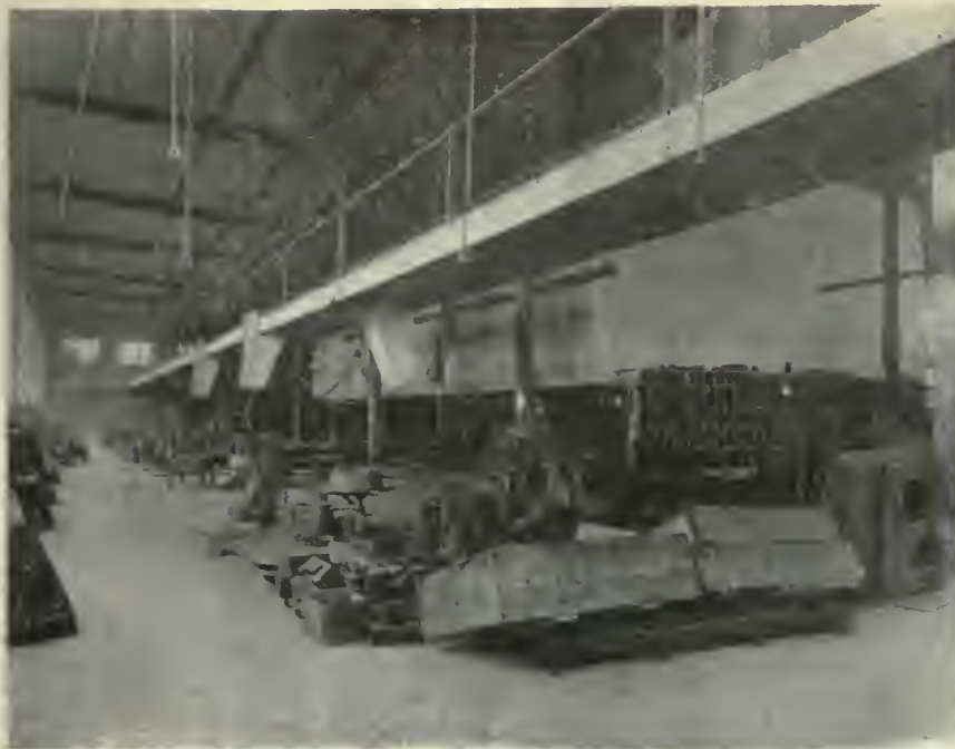
FIG. 6—CORE ROOM AND OVENS, SHOWING OVERHEAD CONVEYORS AND CHUTES FOR DELIVERING CORE SAND FROM SAND MIXER AT THE LEFT.
