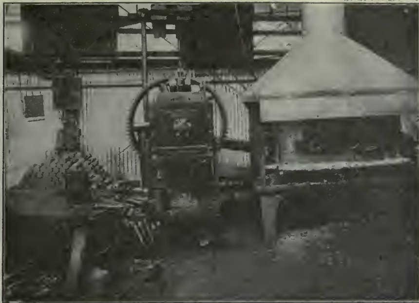
FURNACE AND PRESS FOR CLOSING IN OPEN END AND FORMING NOSE.
