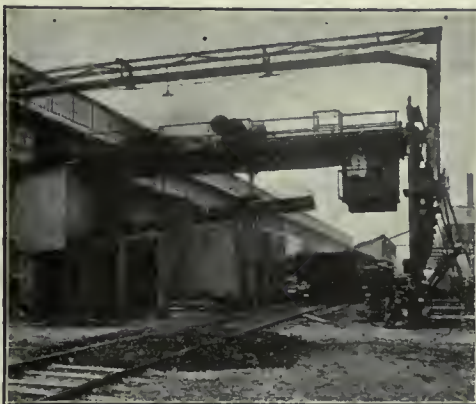
Fig. 1 is a view of the charging end of No. 1 Heating Furnace together with the Electric Overhead Travelling Crane serving it. The slabs are picked up by this Crane by means of a magnet and placed on the akids in front of the Massive Pushers. These machines are of unusually heavy design and are electrically controlled and operated. As hot slabs are drawn for rolling, cold ones are pushed into the furnace at the rear or charging end. Fig. 2 shows a partial end and side view of the No. 1 Heating Furnace with a portion of the Mill Approach Table, Roller Table and of the delivery end of the Slab Transfer in the foreground. Above the top of the furnace may be seen the pipes through which is conveyed the air and powdered coal, by means of which the furnace is heated.
