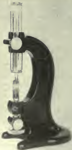
MINIMETER WITH STAND FOR MEASURING THREADS UP TO 80-MM.
