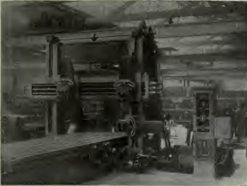
FIG. 2—AN ENGLISH 5-FT. SQUARE PLANER FITTED WITH ELECTRIC DRIVE. INTERIOR OF MACHINE SHOP.
