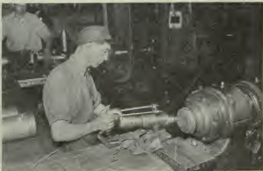
RIVETTING BASE PLATE WITH AIR HAMMER
