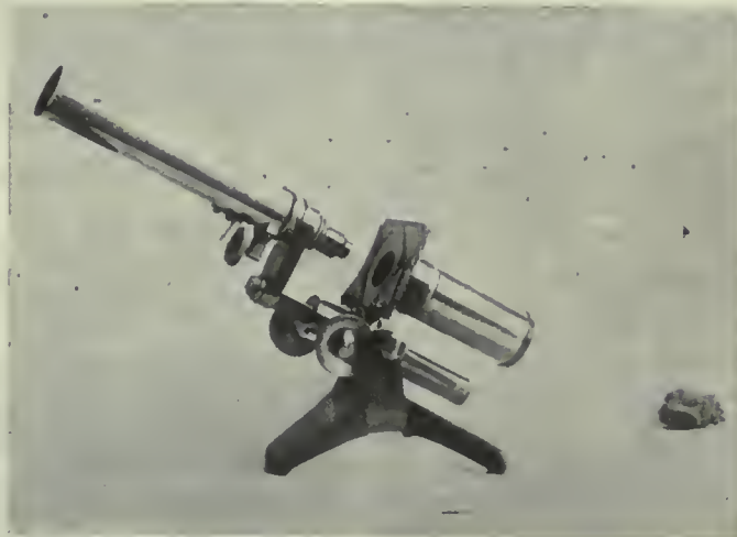
FIG. 2—MICRO-TELESCOPE WITH SHORT FOCUS ATTACHMENT FOR OBSERVATIONS AT CLOSE RANGE, 12 IN. TO 3 FT.
