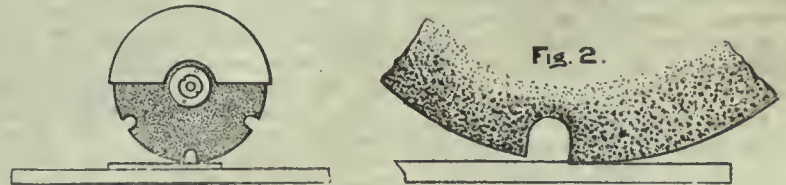
FIGS. 1 AND 2—THE USE OF NOTCHED EMERY WHEELS.
