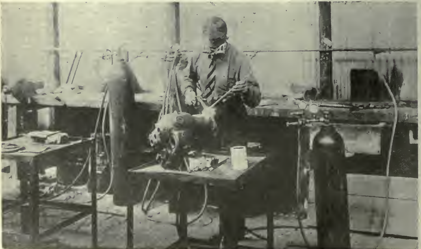
WELDING CAST-IRON AUTOMOBILE ENGINE CYLINDER—BUILDING UP BROKEN FLANGE
