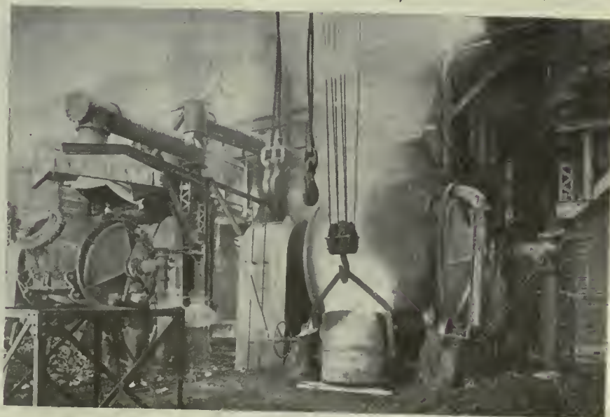
POURING BLISTER COPPER FROM A CONVERTER INTO THE CASTING LADLE AFTER SEPARATION FROM THE NICKEL
