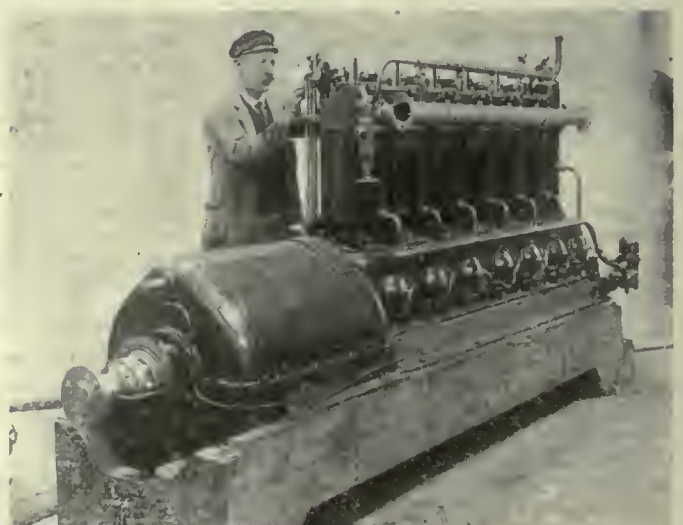
DIESEL ENGINE WITH S K F THRUST BEARINGS FOR PROPELLOR THRUST.
