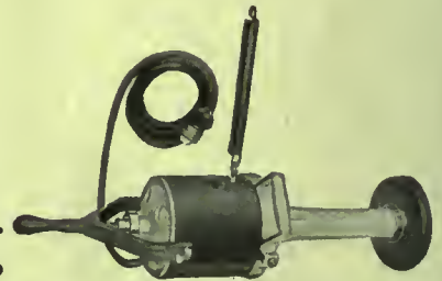
HAND AERIAL GRINDER For cleaning castings or surface work of any kind. Made in four sizes, ¼ to 2 H.P. Weight from 18 pounds up. Guaranteed for hard usage.
