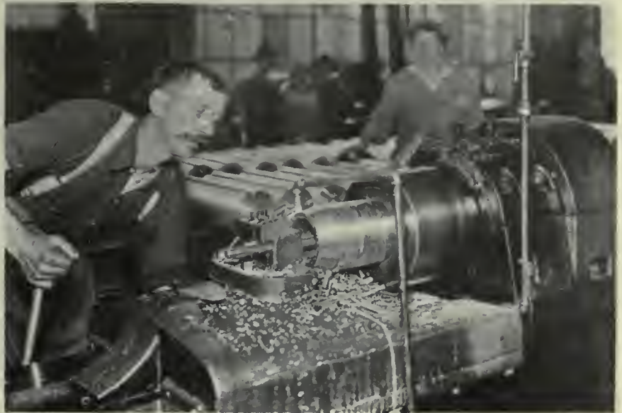
FORMING CHAMFER ON OPEN END OF 6-INCH SHELL
