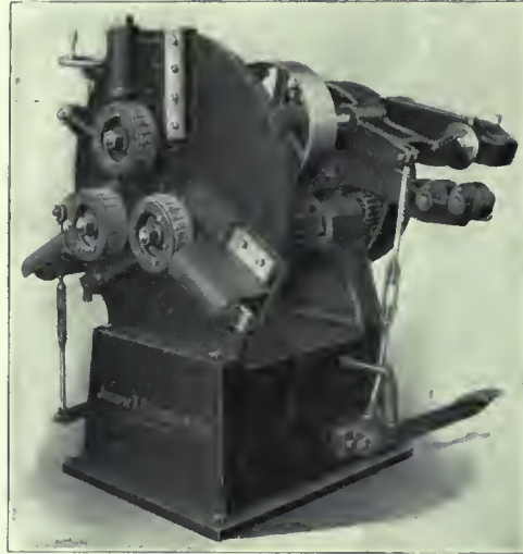
A Universal Machine for cutting and cleaning from 1½" to 6½" flues.
