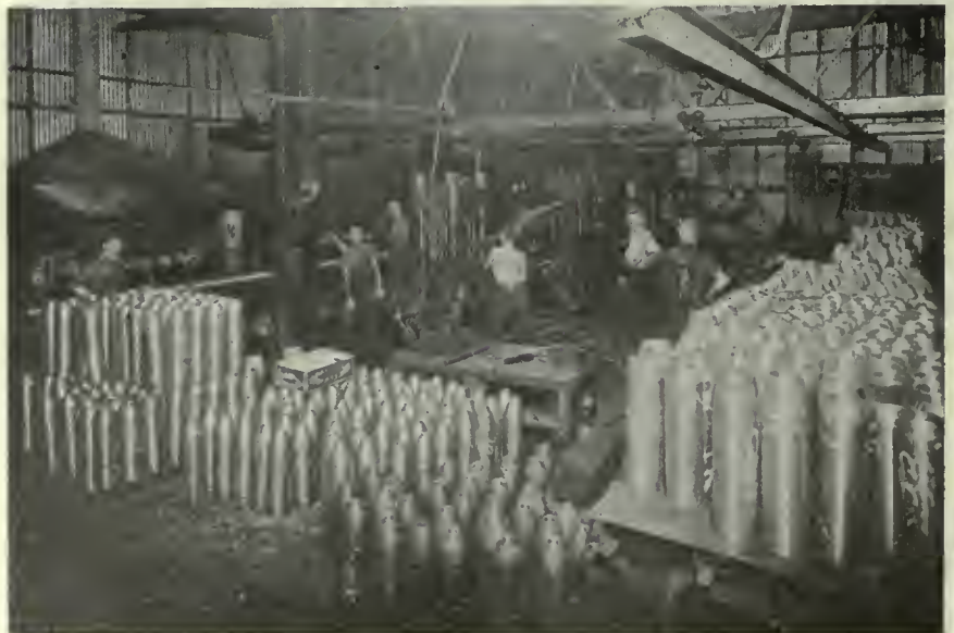
FURNACES AND PRESSES FOR CLOSING IN OPEN END AND FORMING NOSE OF SHELL
