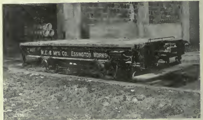
STORAGE BATTERY TRUCK FOR INTER-SHOP AND YARD WORK.
