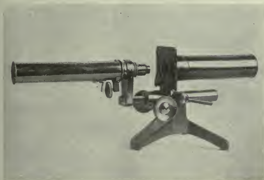
FIG. 1—MICRO-TELESCOPE FOR OBSERVATIONS 6 FT. TO INFINITY.
