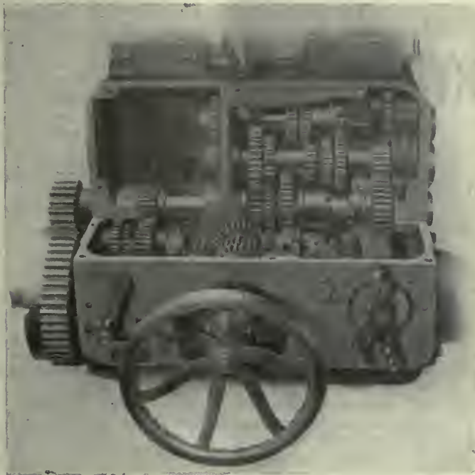
GEAR BOX WITH COVER REMOVED SHOWING MECHANISM.
