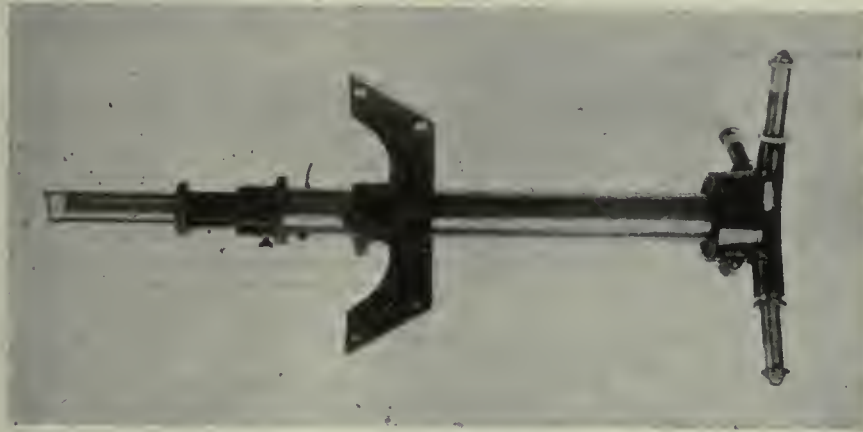
MINIMETER WITH TUBE FOR INSIDE MEASUREMENTS BETWEEN 175-150-MM. AND OF LARGE DEPTHS
