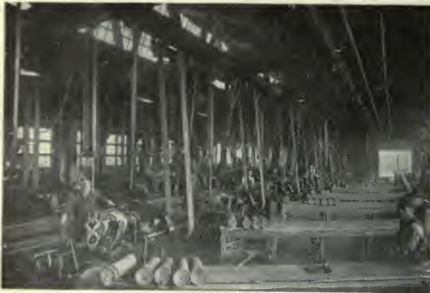
VIEW IN CUTTING AND BREAKING SHOP SHOWING CUTTING-OFF MACHINES, MARKING TABLES AND PNEUMATIC HOISTS
