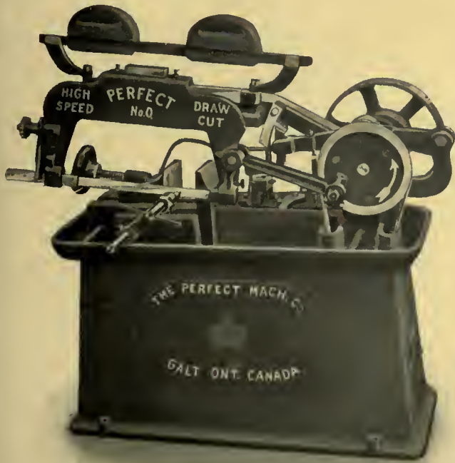
No. 0 PERFECT HIGH SPEED HACK SAW Capacity 0" to 5". Blades 10" to 14". Permanent or Swivel Vise. A real machine tool with the latest improvements. Worth investigating.
