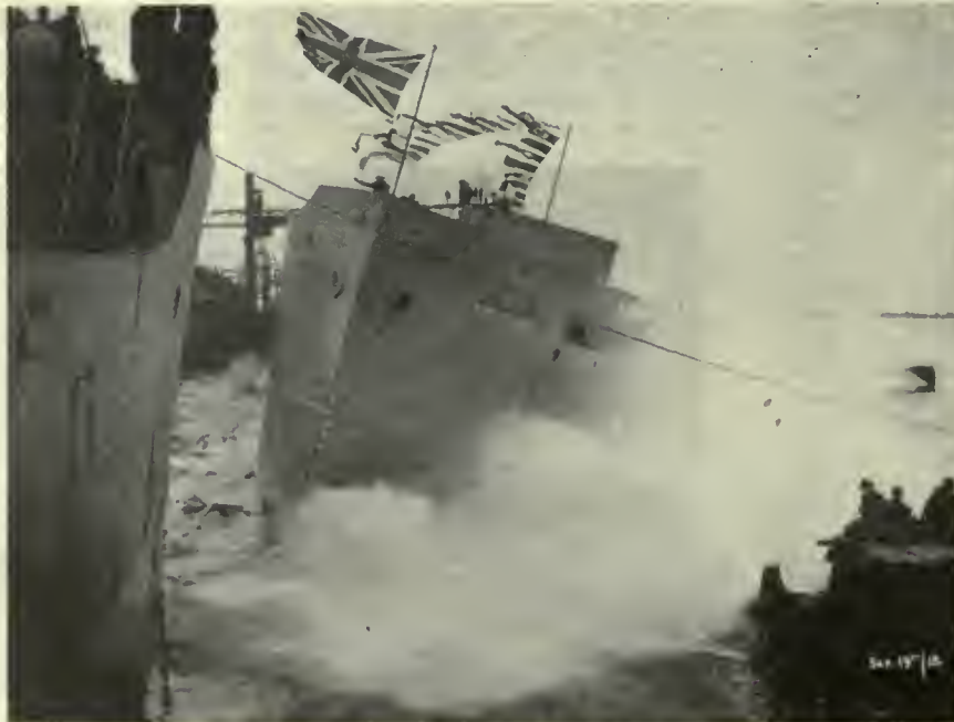
LAUNCHING A 3,500-TON STEEL SHIP
