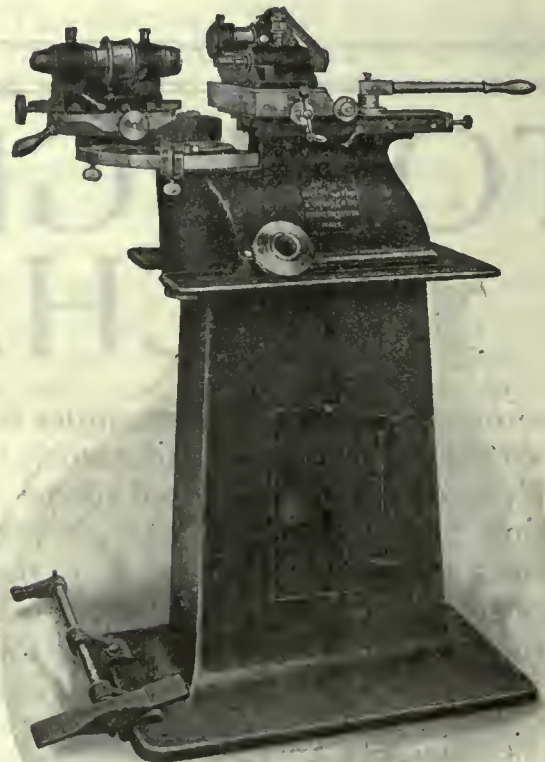
The Rivett No. 205 Hand Operated Radial Grinder 7" swing. Grinding capacity up to 4" dia. Grinding capacity up to 2" radius. This machine is designed for spherical surfaces as well as ball races, ball and socket joints, etc. All adjustments to grind are easily and quickly made.
