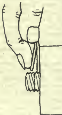
FIG. 5—IMPROVED WAY TO INSERT COTTER
