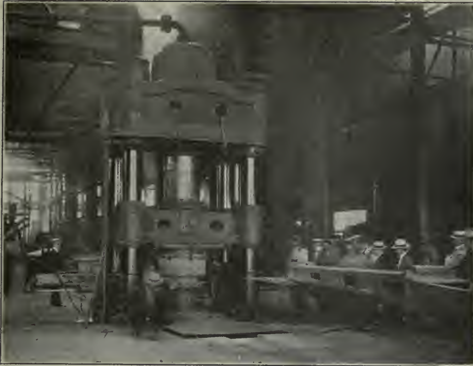
2,000-TON STEAM INTENSIFIER FORGING PRESS, FORGING INGOT INTO TYRE BLOOM
