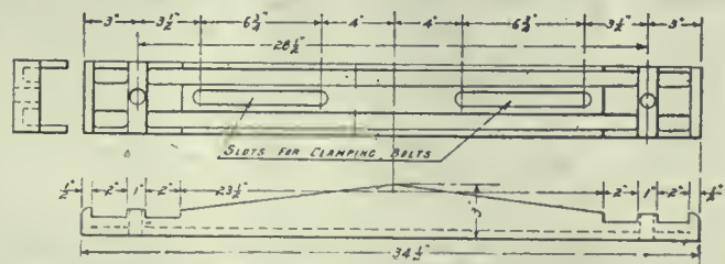
FIG. 18—CAST IRON MOTOR OR SHAFT HANGER SUPPORT TO SPAN ACROSS TWO CHANNEL GIRDER (THIS IS AN EXAMPLE OF AN ISOMETRIC DAAWING FOR WHICH THREE VIEWS ARE NECESSARY.
