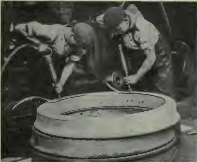
FIG. 2—ENGLISH PNEUMATIC TOOLS IN SERVICE CHIPPING RAILROAD TIRES AT THE BOLTON IRON AND STEEL PLANT.
