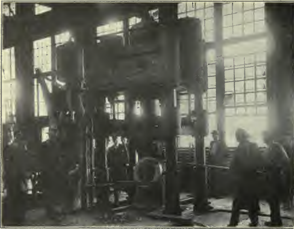
6,000-TON STEAM INTENSIFIER HYDRAULIC BECKING PRESS, FORGING BLOOM INTO ROUGH OUTLINE OF TYRE
