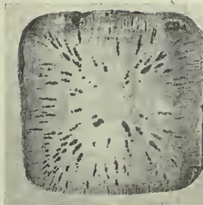
No. 2—Section of electric steel ingot showing (1) blowholes (wild steel); (2) lappiness, or folds in the ingot; (3) included unfluxed fire clay.
