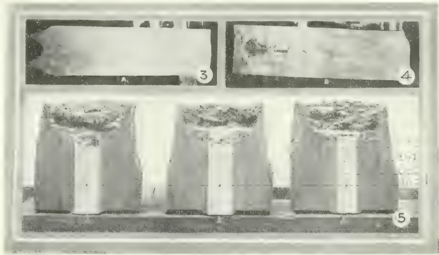
Fig. 3. Ingot made by "Hadfield" process; perfectly sound, free from blow holes, piping and segregation. Fig. 4. Ingot made in ordinary manner; unsound, having blow holes, piping and segregation. Fig. 5. Upper portions of three ingots made by the "Hadfield" process.
