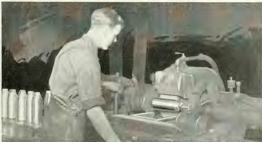
GRINDING SHRAPNEL. ALOXITE WHEEL ON A FORD SMITH MACHINE
