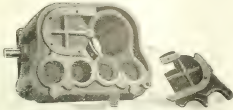
Broken Cylinders Before Welding
