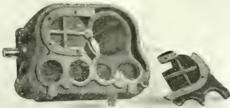
Broken Cylinders Before Welding
