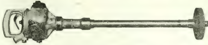
The cut illustrates our No. 7 "LITTLE DAVID" Grinder, fitted with 21" Extension Shaft, housing and outer bearing. The grinding wheel is 6" x 1", of composition suited to the work, and its free speed is 3,000 r.p.m. Weight 24 lbs.
