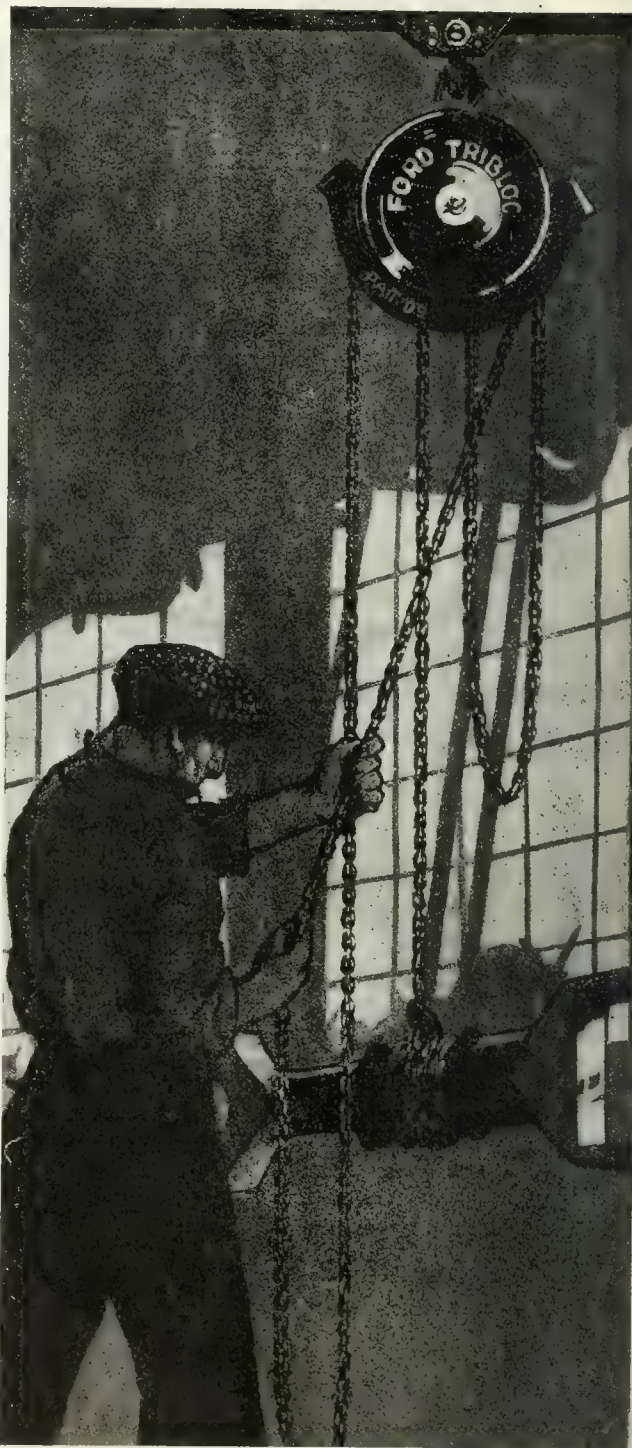
The Chain Hoist in the Foreground of Service
