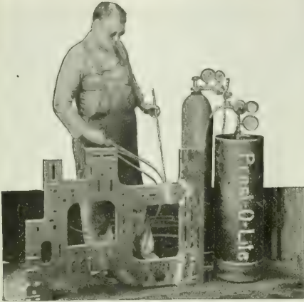
Operator repairing broken loom by the Prest-O-Lite Process of Oxy-Acetylene Welding.
