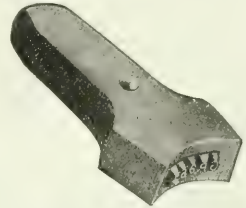
Special "Champion" holders with type chamber curved on face for marking sides of shells.
