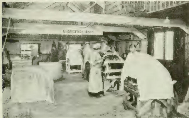
CONSTRUCTING AEROPLANE NOSES WITH WOMEN WORKERS. Illustration, Courtesy Engineering.
