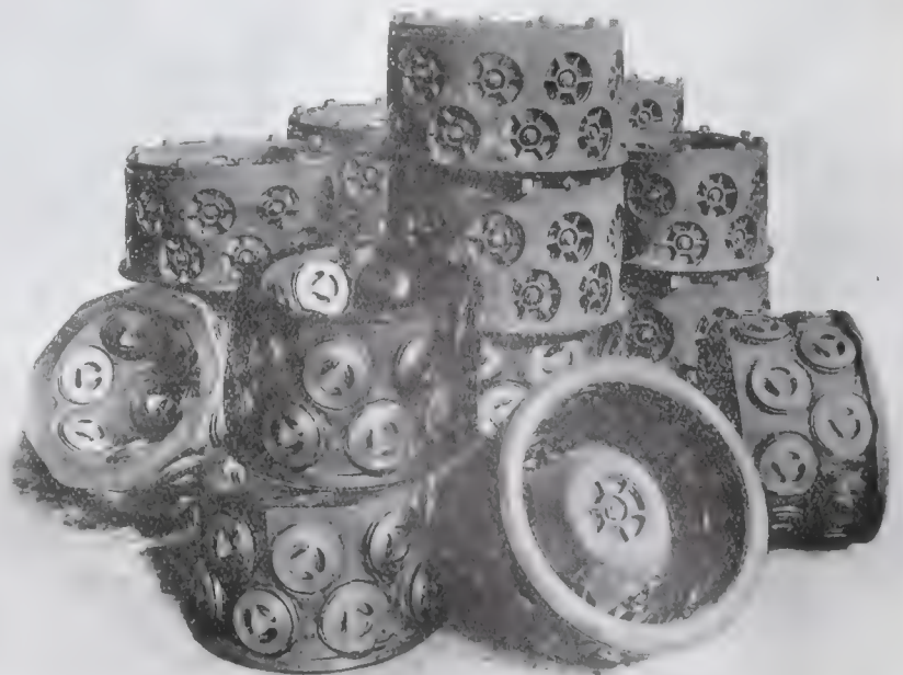
FIG. 1. PLATE VALVES ARRANGED IN CAGES TO REPLACE LARGE POPPET VALVES PREVIOUSLY EMPLOYED.
