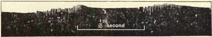
FIG. 17.—The Syllables "pop-op-op" Spoken near a Battery of Five Telephones in series. Plate moving more slowly. (Enlarged).*
