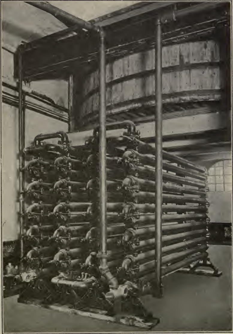
FIG. 175.—SCHNEIBLE'S HOT BEER COOLER, COLD WATER SECTION.
