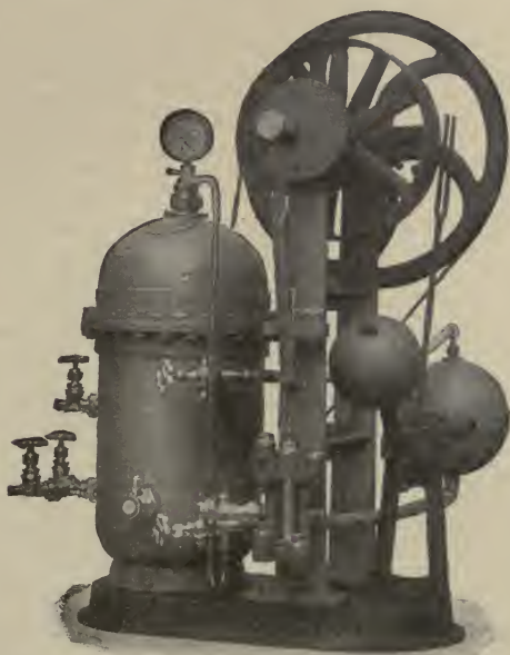
FIG. 136.—POWER-DRIVEN CARBONATOR—AMERICAN SODA FOUNTAIN COMPANY'S TYPE.
