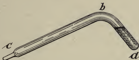
FIG. 45.—TUBE FOR LIQUEFYING \text{CO}_2 .
