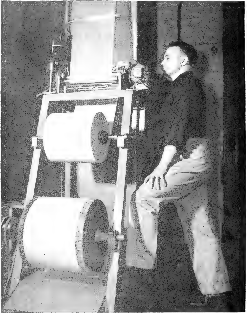
A forest-products researcher inspecting paper sheets as they go through a machine to be made into "papreg," a paper plastic developed at the Forest Products Laboratory, Madison, Wis.
