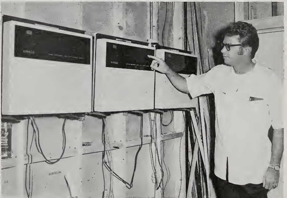
These three Store and Forward Modules are self-contained magnetic tape units. They store transactions and forward them to the central computer when polled by telephone.
