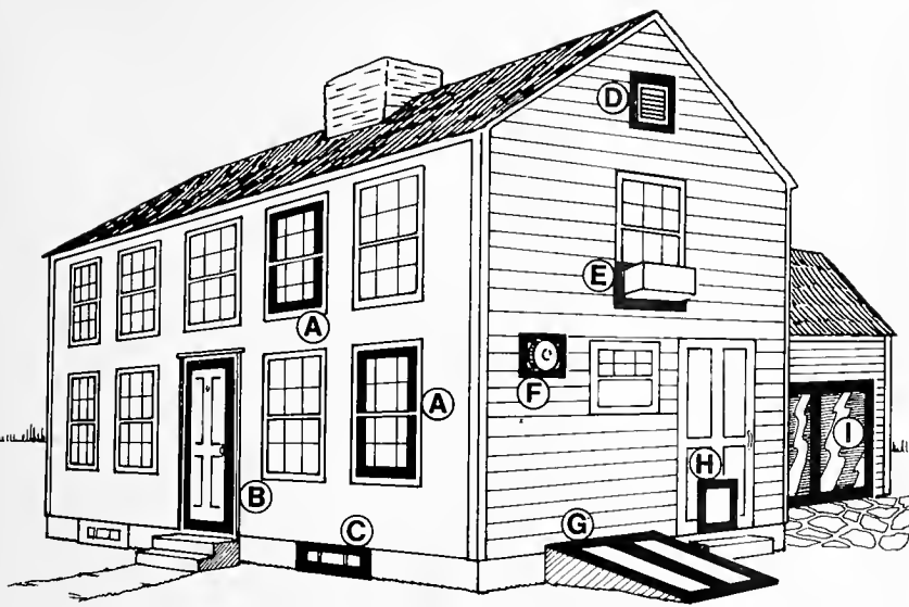
Areas to caulk and weatherstrip: Windows (A), doors (B), cellar casements (C), attic vents (D), air conditioners (E), kitchen fans (F), basement bulkheads (G), pet entry doors (H), and garage doors (I).—Diagram courtesy of the Schlegel
