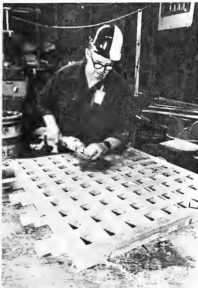
Workleaderman John Rylee smooths a section of the grating prior to assembly.
