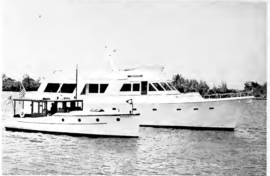
A photo exhibit in 1982 at The Haggin Museum in Stockton, Calif., on Stephens Pleasure Craft dubbed this photo "The Oldest and Newest." The 1925 Graceta, 36 feet by 11 feet by 3 feet, 125 horsepower, is shown next to the 1982 Iwone, 74 feet by 18 feet by 4.6 feet, 1300 horsepower, revealing the contrasts in products of the Stephen Yard over nearly six decades. The Graceta is a familiar sight in Stockton waters; the Iwone was shipped to Hong Kong.
