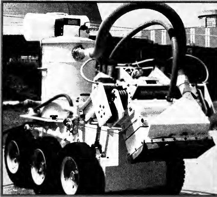
"The Moose," a first-of-a-kind working robot designed for Electric Power Research Institute, was built to work in the hostile environment of the Three Mile Island nuclear power station to remove protective coatings and break up radioactive concrete. The Moose can deliver 1200 hammer blows per minute.
