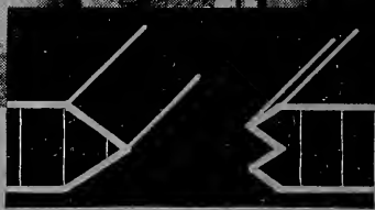
The exclusive Celotex Double-A lock joint, reversible and interlocking, anchors every piece without batten strips.
