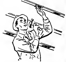
Nail Upson Fasteners to furring strips, 8' apart.
