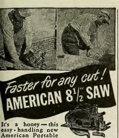
Electric Saw! Balanced for one-hand operation. Cuts fast in any position... for wood, stone, tile, sheet metal, compositions. Big power G.E. motor develops 2 1/8 H.P. Big capacity blade will cut a 2 1/8" plank at 45°, or 3" straight cut. Blade speed 5300 R.P.M. Wide base calibrated for ripping. Holds accurate depth of cut and angle adjustment. Write for details and FREE demonstration.
