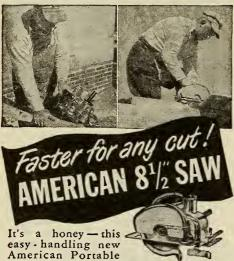
Electric Saw! Balanced for one-hand operation. Cuts fast in any position... for wood, stone, tile, sheet metal, compositions. Big power G.E. motor develops 2 1/8 H.P. Big capacity blade will cut a 2 1/8" plank at 45°, or 3" straight cut. Blade speed 5300 R.P.M. Wide base calibrated for ripping. Holds accurate depth of cut and angle adjustment. Write for details and FREE demonstration.
