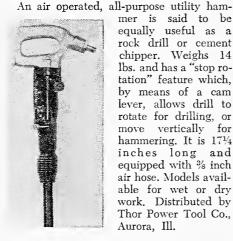
mer is said to be equally useful as a rock drill or cement chipper. Weighs 14 lbs. and has a "stop rotation" feature which, by means of a cam lever, allows drill to rotate for drilling, or move vertically for hammering. It is 171/4 inches long and equipped with % inch air hose. Models available for wet or dry work. Distributed by Thor Power Tool Co., Aurora, Ill.
