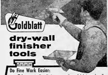
Trio practically eliminates sanding af joints and nail spots. This 3-in-1 tool shears, feathers, and finishes with 3 interchangeable blodes: 11" x 4" concave shearing curve; 11" x 4" straight working edge; 8" x 4" cancave shearing edge. Comfortable plastic handle. Order No. Trio, complete with high carbon spring steel blades, \$4.95. With rust-resistant stainless steel blades, \$5.95.
