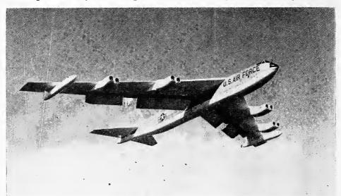
The Strategic Air Command's first all-jet heavy homber, the Boeing-built B-52 Stratofortress, on May 20, 1956, became the first U.S. aircraft to air-drop a hydrogen bomb. The B-52 Stratofortress eventually will replace the B-36. It has a 185 foot wingspan, but, despite this great size, its eight jet engines place it in the 650 mile per hour speed class. It has a ceiling of more than 50,000 feet and a range of over 6,000 miles without refueling, and it can be refueled in flight.
