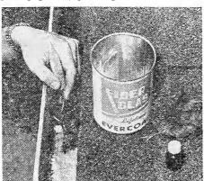
or just about any other material — stone, wood or metal. Plastic material sets in 20 to 30 minutes and is completely waterproof. Developed by Fibre Glass-Evercoat Co., 7220 Vine St., Cincinnati, Ohio.
