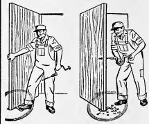
Holds door firmly while you work . . . just step on it, pull door over it, step off and the door won't move.
