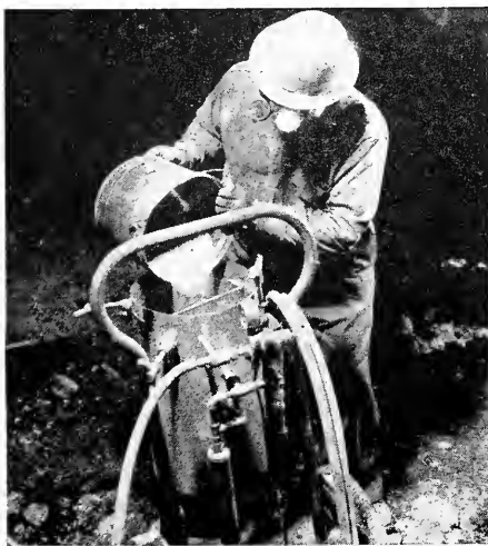
An Oxweld Powder Dispenser is used in powder-lancing to deliver the required amounts of powder at a uniform, accurately controlled rate. The dispenser's powder capacity is 200 lbs.
