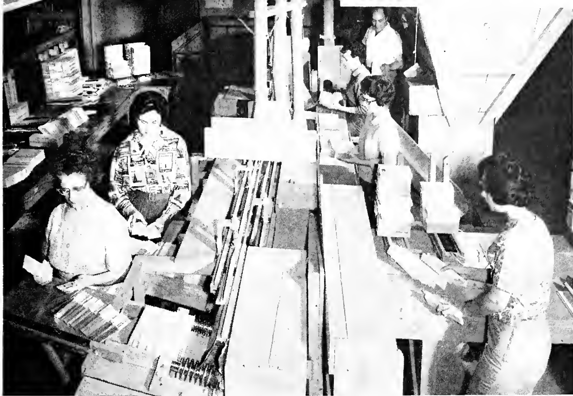
Blocks cut from sized blanks are fed into the sawing machine, which spits out slats. Women members of Local 3036 perform an initial sort.
