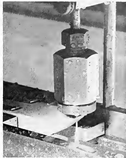
Water jet shooting from the nozzle under 50,000 pounds of pressure per square inch cuts 2-inch maple block.
