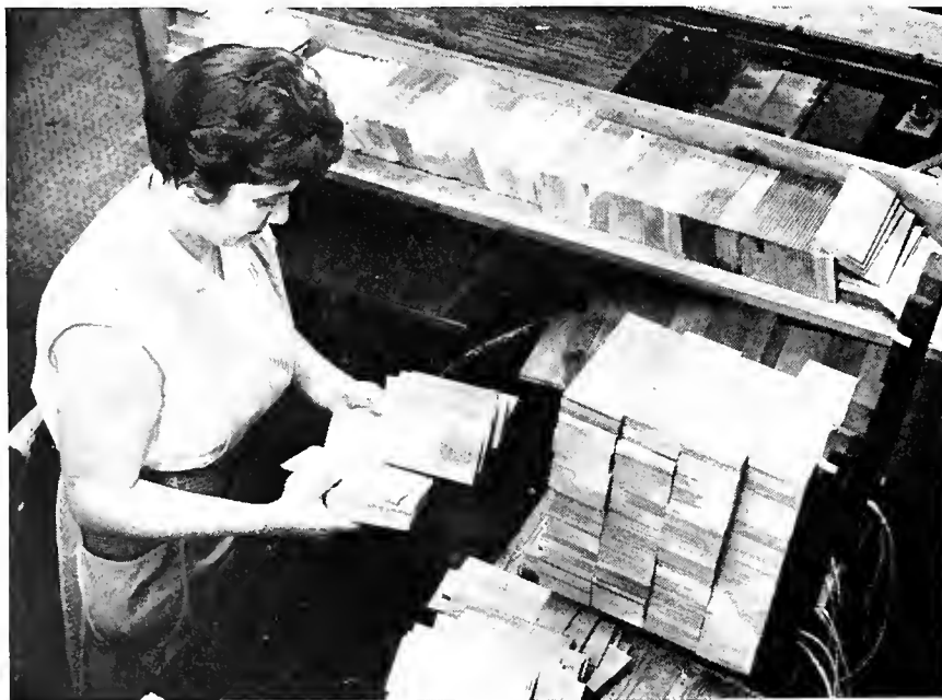
The final sorter (below), checks for defects, grain and color consistency before slats are loaded into the high-temperature retorts for wax and color impregnation.
