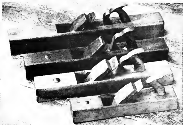
TRYING PLANES , with flat sole and blade for more perfect smoothing. Hollow-grasp handles, such as there appeared in the mid-18th Century. Ranging in size from 28" to 18", the largest was doubtless used as a flooring plane.
