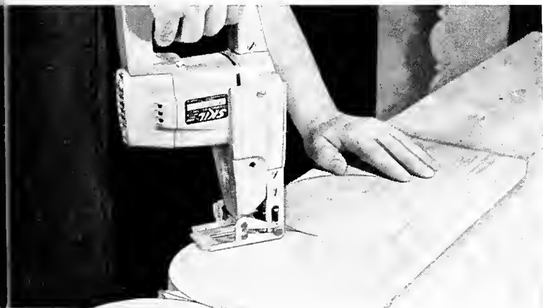
Cuts like a jig saw —makes intricate scroll cuts, pattern cuts and template cuts in wood, metal, plastic, etc.
