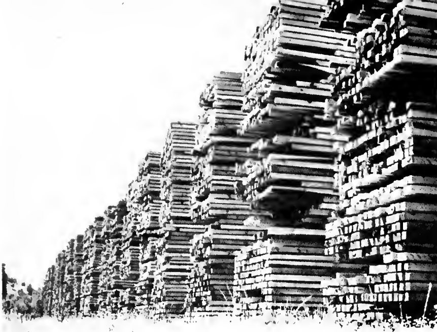
At the sawmill (above), rough blanks are air dried. They then go to the plant in San Leandro, Calif., where the first step is final sizing on the planing mill (below).
