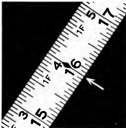
Standard stud spacing. Diamond mark on graduation line designates 16" centers.
