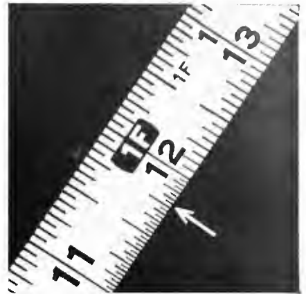
Marked both feet and inches. First 12 inches, bottom edge, to 32nds inch.
