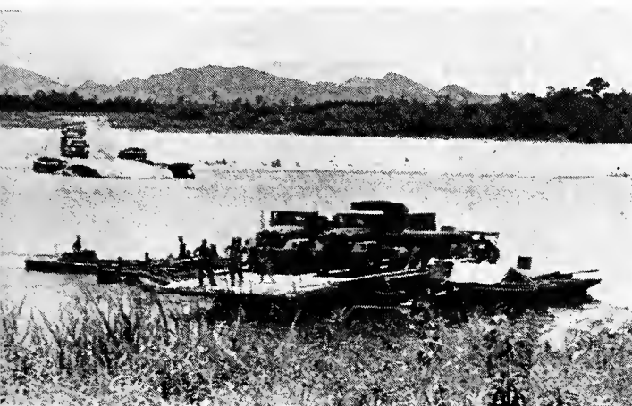
SOON TO BE OBSOLETE —This Marine Corps ferry, which transported 15 vehicles a day across the Thu Bon River, was replaced by the bridge.
