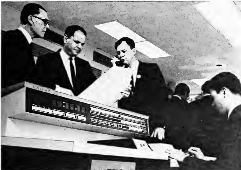
PUNCH-CARD VOTING —A single UNIVAC 1108 computer tabulated and analyzed returns from about two million student punched card ballots (such as the one shown at right) during Choice 68, a "national collegiate Presidential primary" last April 24. The computer, located in the Washington, D.C. offices of Sperry Rand's Univac Federal Systems Division, made the first complete breakdown in history of voting preferences of an entire nationwide group of the U.S. population. Choice 68 was co-sponsored by Time Magazine and the Univac Division of Sperry Rand Corporation.
