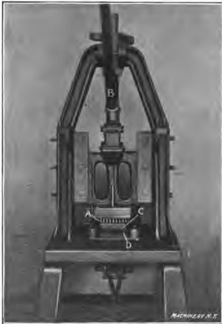
Fig. 15. Hand Loading Machine for Loading the Cartridge
