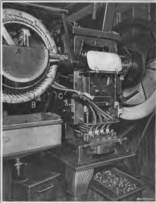
Fig. 6. Drawing Press used for First, Second, and Third Redrawing Operations—Four Cups per stroke at the Rate of 24,000 per Hour
