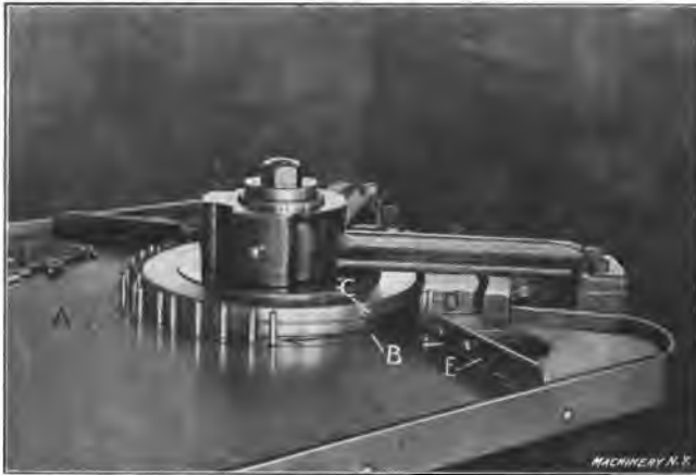
Fig. 17. Cannelluring Machine for Forming the Grooves in the Bullet
