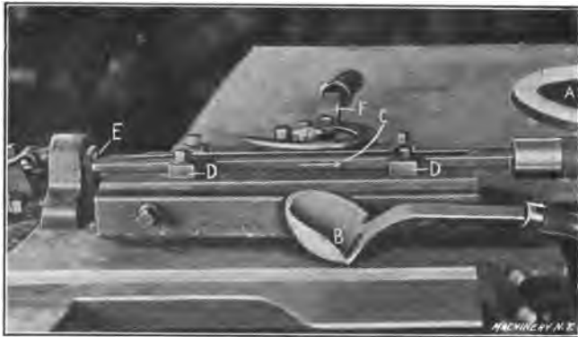
Fig. 11. Molds in which the Slugs for the Bullets are Cast
