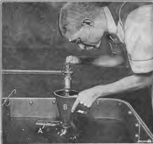
Fig. 4. "Spouting" a Redrawing Die—Hardening the Hole and Leaving the Exterior Comparatively Soft
