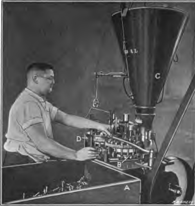
Fig. 2. Inserting the Powder and Bullets and Crimping— Loading 0.30-caliber Cartridges
