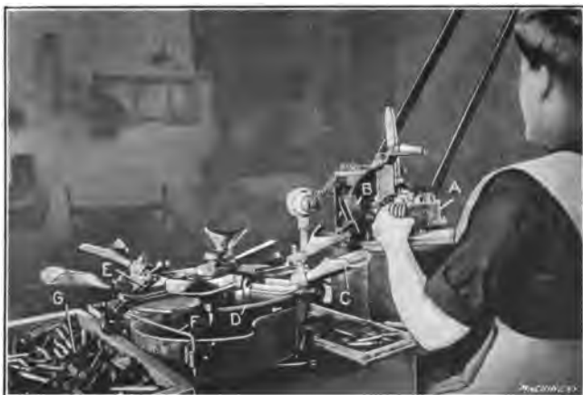
Fig. 8. Inspecting and Weighing 0.30-caliber Cartridges
