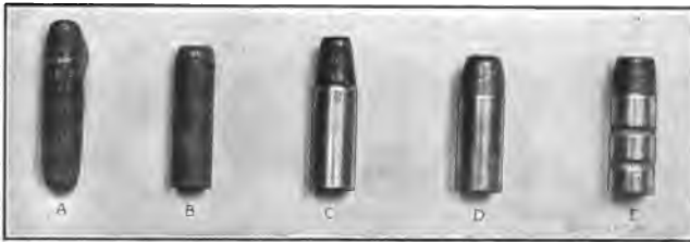
Fig. 14. Operations performed on the Lead Filling before and after Assembling in the Metal Case
