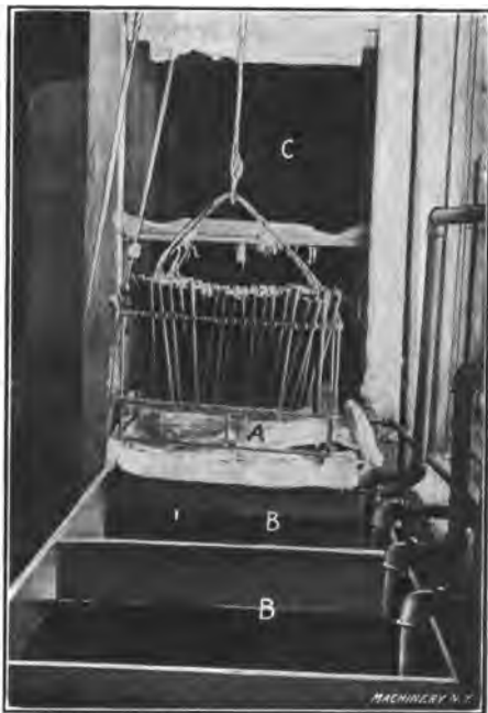
Fig. 7. Waterproofing Tanks and Drying Cupboards
