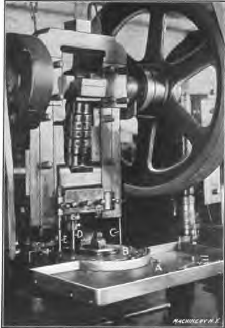
Fig. 16. Swaging Machine for Forming the Lead Filling and the Metal Case to the Desired Shape
