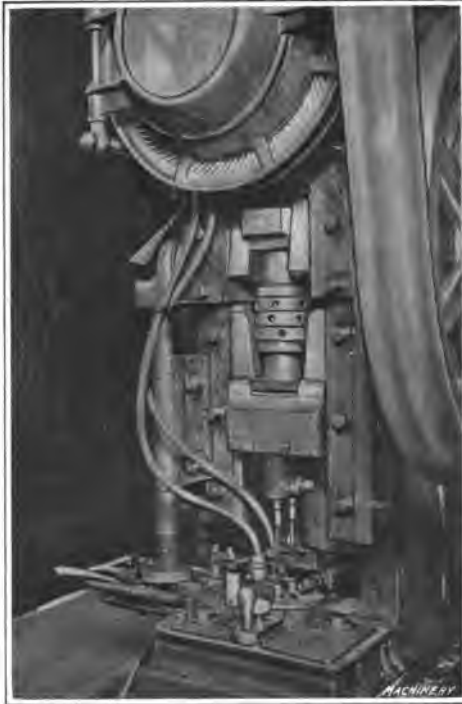
Fig. 2. Type of Drawing Press used for Redrawing Nickel Jackets for Spitzer Bullets using Two Punches and Dies
