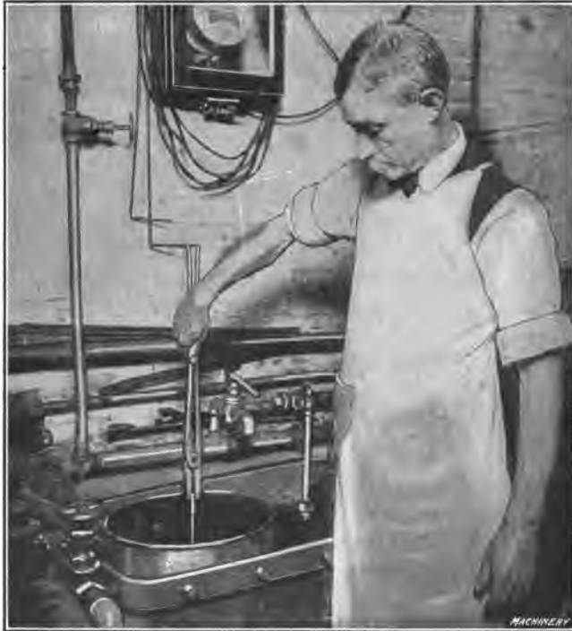
Fig 6. Hardening a Redrawing Punch—Note Method of Dipping
