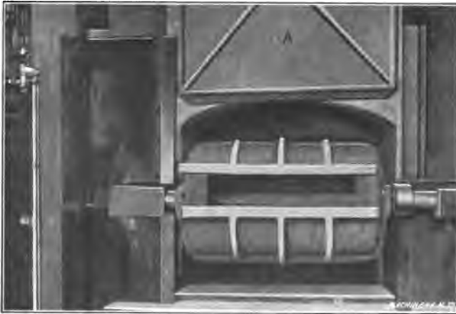
Fig. 1. Cylindrical Drum in which the Cups are Annealed
