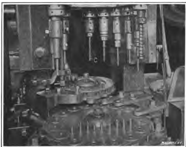
Fig. 6. Machine used for Forming the Nickel Cases for Spitzer Bullets and Assembling the Lead Fillings in them
