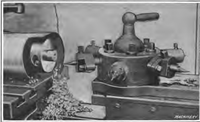
Fig. 12. Making the Pointing Die for a Spitzer Bullet in a Hand Screw Machine
