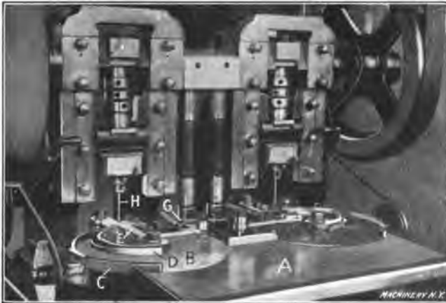
Fig. 4. Double-headed Friction-dial Drawing Press used for the Various Drawing Operations
