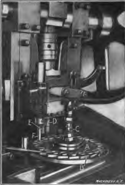
Fig. 12. Expanding Machine for Partially Forming the Head on the Brass Cap
