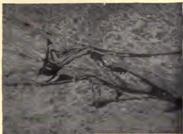
NO. 60. SLAG AT CENTER OF TREAD.
