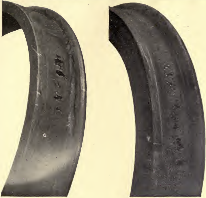
SHELLED-OUT STEEL TIRE AND WHEEL,
