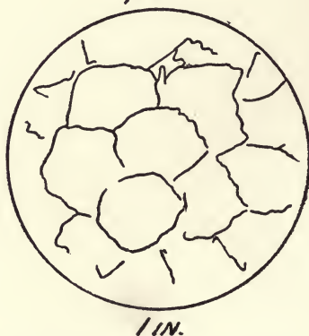
INTERPRETATION OF GRAIN STRUCTURE IN SCHOEN WHEEL AT VARYING DISTANCES BELOW SURFACE OF TREAD.
