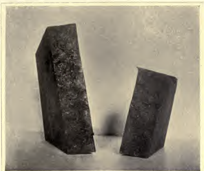
BURNED METAL OF SCHOEN STEEL WHEEL
