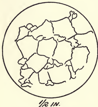
INTERPRETATION OF GRAIN STRUCTURE IN SCHOEN WHEEL AT VARYING DISTANCES BELOW SURFACE OF TREAD.
