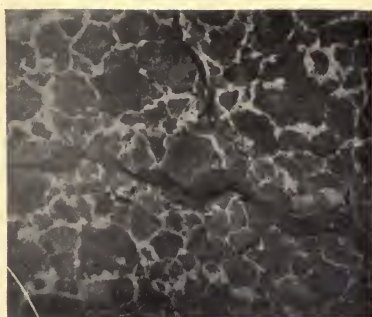
NO. 62. SLAG \frac{1}{4} IN. BELOW SHELLLED OUT SPOT
