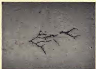
No. 50. SLAG FLAW NEAR EDGE OF SOLID METAL.
