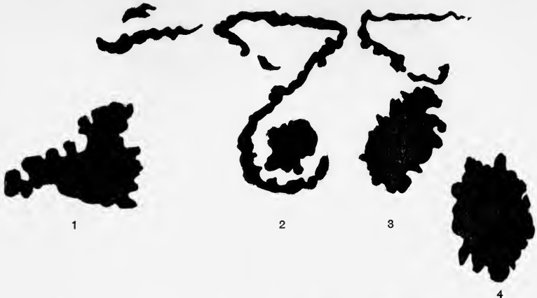
CONTACTS OF 33-INCH WORN CAST IRON WHEEL UNDER GONDOLA CAR. WEIGHT ON WHEEL, 14,575 LBS.
