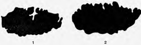
CONTACTS OF 78-IN. STEEL-TIRED DRIVING WHEEL, ATLANTIC LOCOMOTIVE. WEIGHT ON WHEEL, 19,995 LBS.
