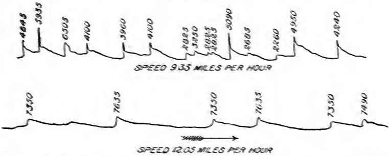
EXAMPLES OF LATERAL THRUST REGISTRATIONS OF LOADED COAL TRAINS, WITH CARS OF 100,000 LBS. CAPACITY.
