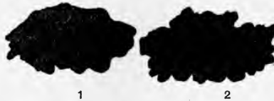
CONTACTS OF 48\frac{5}{16} -IN. STEEL-TIRED TRAILER TRUCK WHEEL, ATLANTIC LOCOMOTIVE. WEIGHT ON WHEEL, 19,210 LBS.
