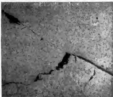
NO. 54. SLAG \frac{1}{4} IN. BELOW TREAD IN SOLID METAL.
