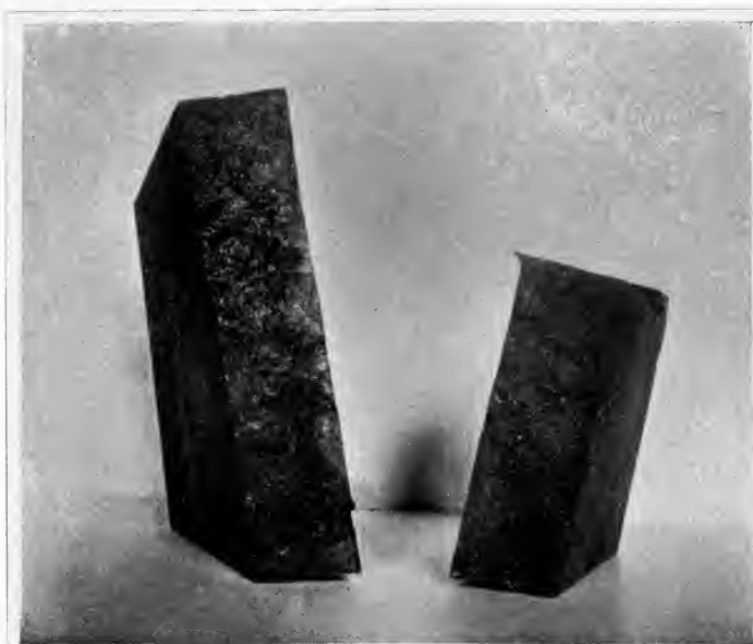
BURNED METAL OF SCHOEN STEEL WHEEL
