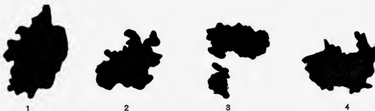
CONTACTS OF 35-IN. STEEL-TIRED WHEEL UNDER CAFÉ CAR. WEIGHT ON WHEEL, 6,075 LBS.
