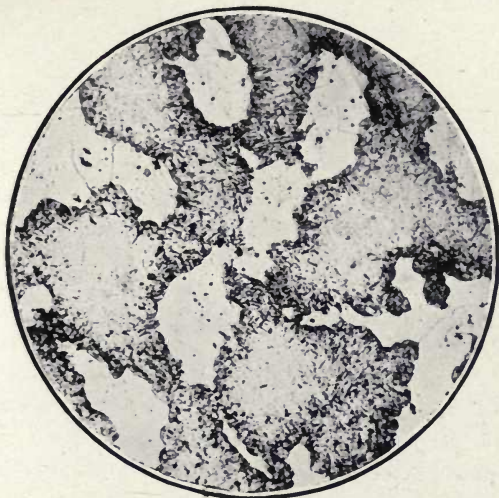
FIG. 35.—Troostite fringes within the core. x 200.
