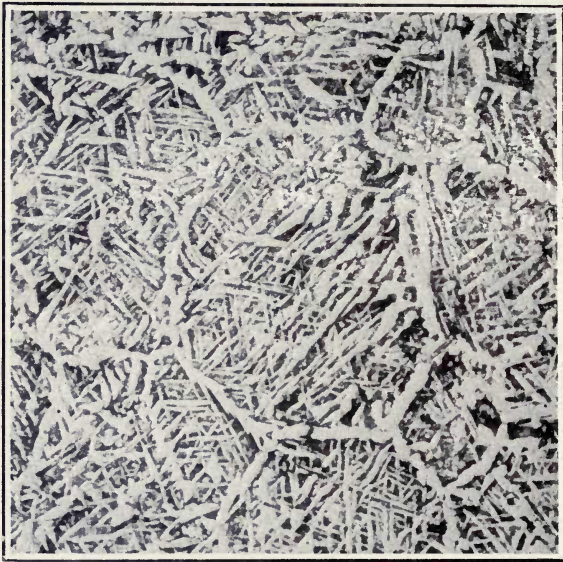
FIG. 3.—Overheated structure of mild steel. x 25.
