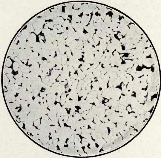
FIG. 50.—Steel which machines well. x 100.
