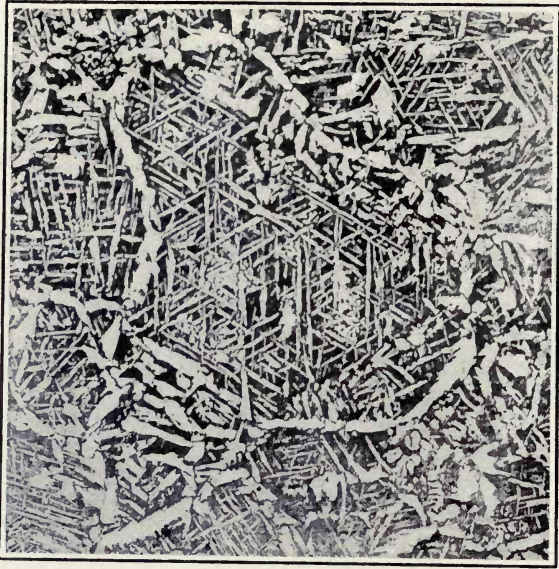
FIG. 5.—Peg quenched at 750° C. on heating. x 25.
