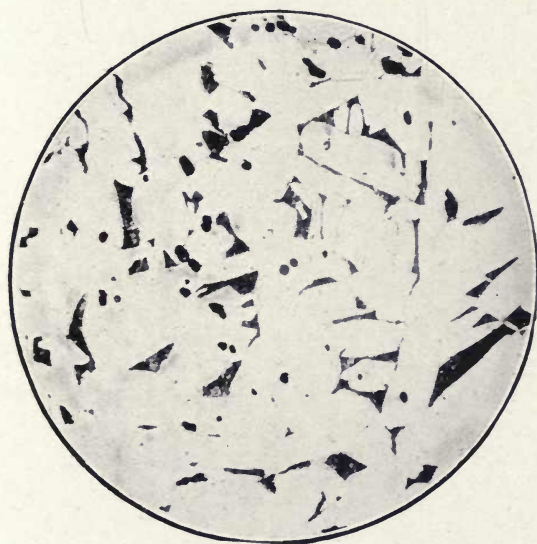
FIG. 51.—Similar steel to fig. 50, which machines badly. x 100.
