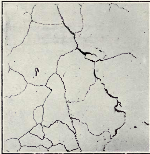
FIG. 29.—Crack proceeding along cementite outlines. \times 100 .
