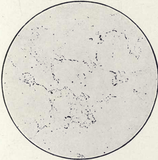
FIG. 46.—Cementite envelopes in slowly-cooled mild steel. x 100.
