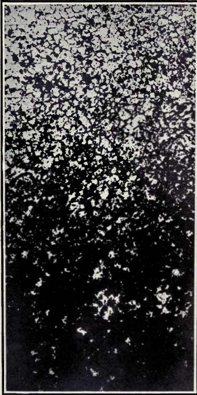
FIG. 34.—Troostite fringe on the edge of soft spots. x 200.
