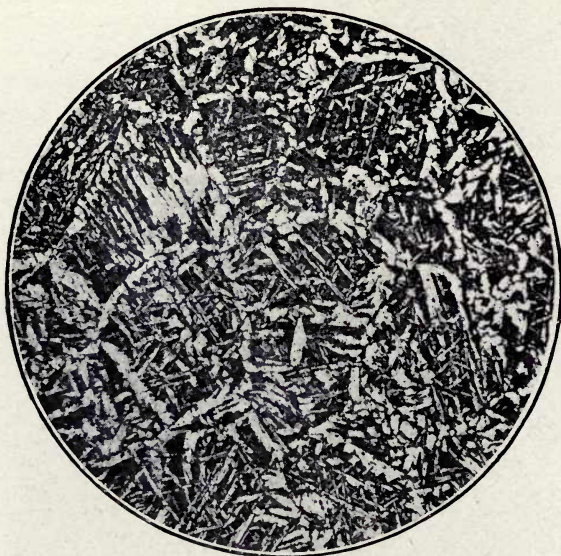
FIG. 8.—Peg quenched at 780° C. on heating. x 25.
