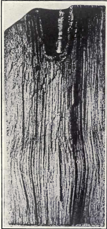
FIG. 32.—Fibrous fracture along length of case-hardened die.
