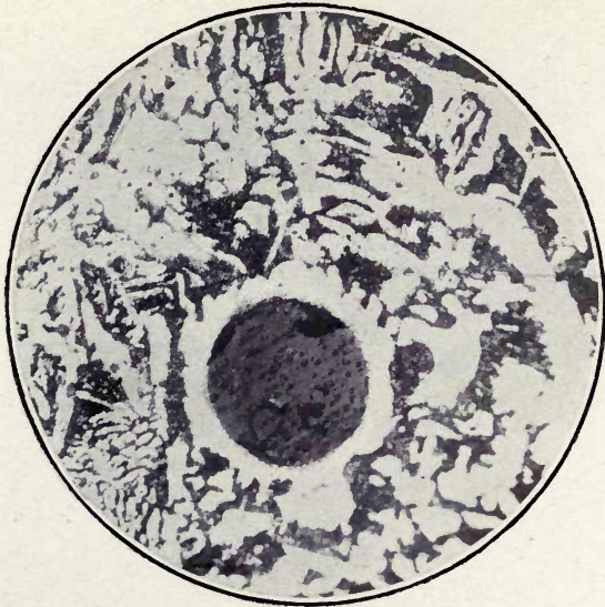
FIG. 25.—Slag globule in ferrite envelope. x 50.
