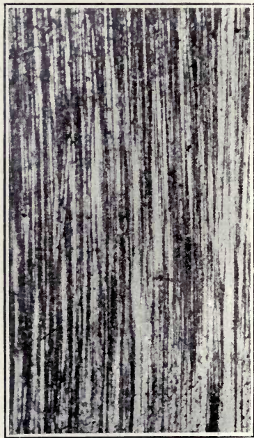
FIG. 37.—Streaky troostite due to grinding. x 25.
