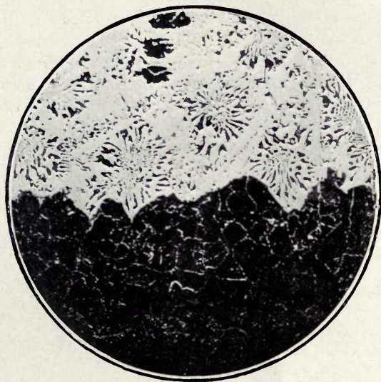
FIG. 61.—Microstructure of phosphide blister.
