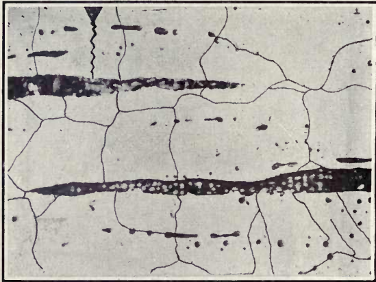
FIG. 23.—Wrought iron containing slag streaks. \times 150 .
