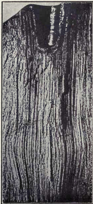
FIG. 32.—Fibrous fracture along length of case-hardened die.
