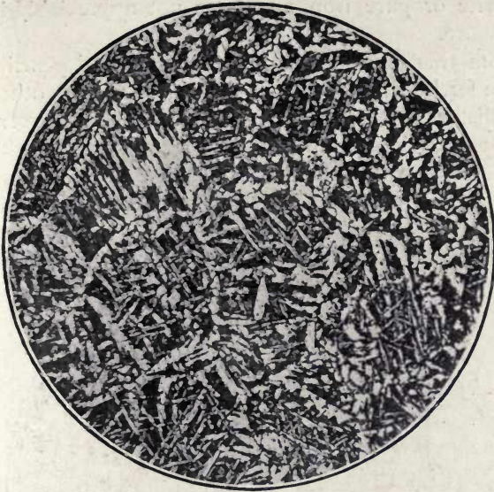
FIG. 8.—Peg quenched at 780° C. on heating. \times 25 .
