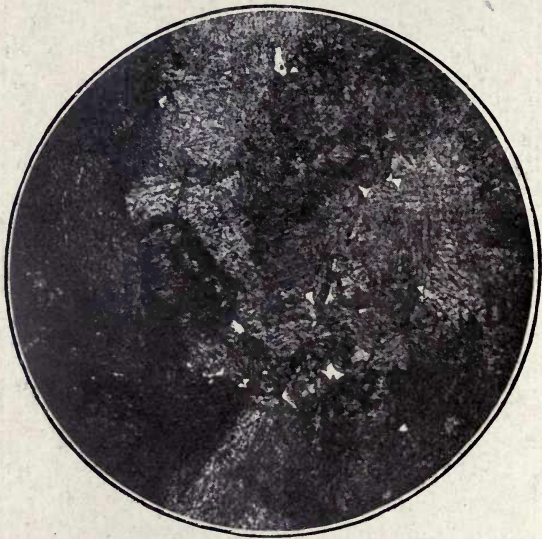
FIG. 12.—Peg quenched at 800° C. on cooling. \times 100 .
