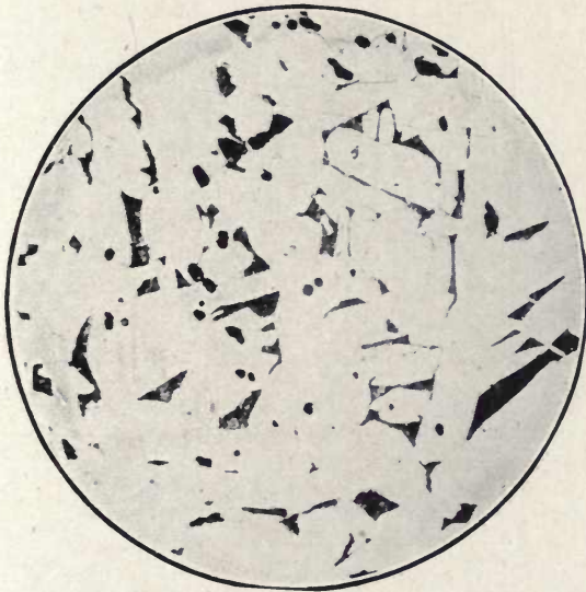
FIG. 51.—Similar steel to Fig. 50, which machines badly. \times 100 .
