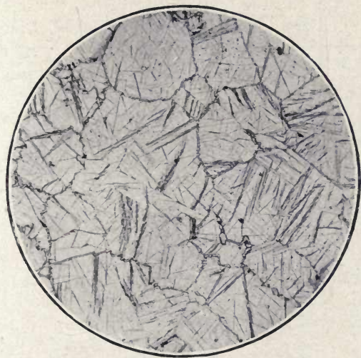
FIG. 30.—Cementite in needles and cell walls in quenched specimen. \times 300 .
