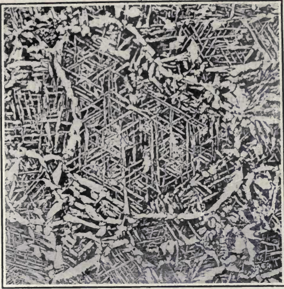
FIG. 5.—Peg quenched at 750° C. on heating. \times 25 .
