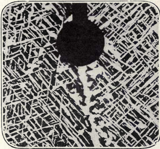
FIG. 65.—Irregular impact figures are obtained from coarsely crystalline material according as the bottom of the notch falls on or on either side of a crystal junction. \times 25 .
