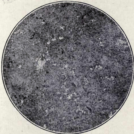
FIG. 9.—Peg quenched at 800° C. on heating. \times 25 .
