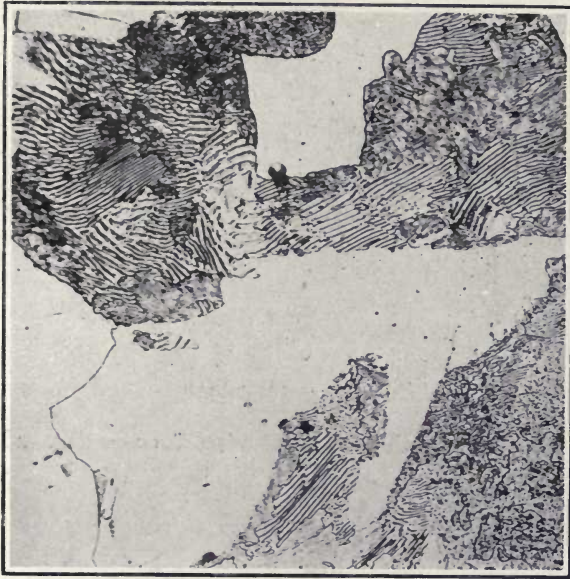
FIG. 15.—Peg quenched at 670° C. on cooling. \times 800 .
