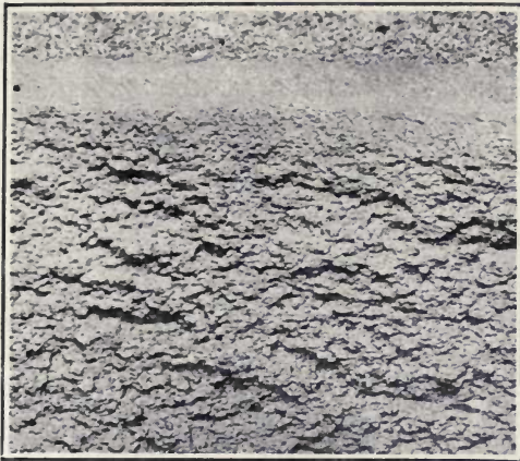
FIG. 27.—Coarse crystalline appearance of fracture due to free cementite.
