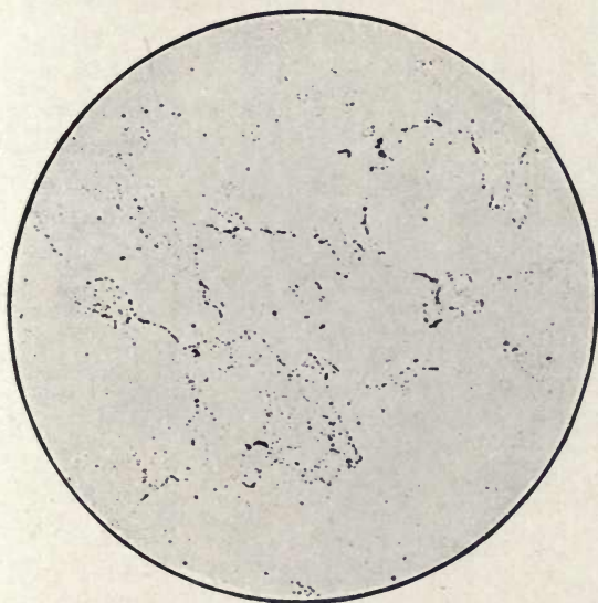
FIG. 46.—Cementite envelopes in slowly-cooled mild steel. \times 100 .
