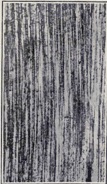
FIG. 37.—Streaky troostite due to grinding. \times 25 .
