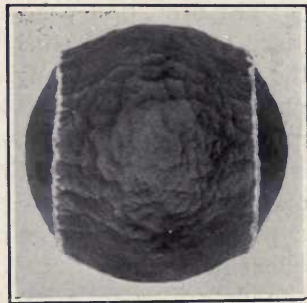
FIG. 93.—Disc of mild steel distorted by repeated quenching.
