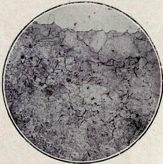
FIG. 44.—Quenched bar with sharply defined carbonless envelope. \times 100 .
