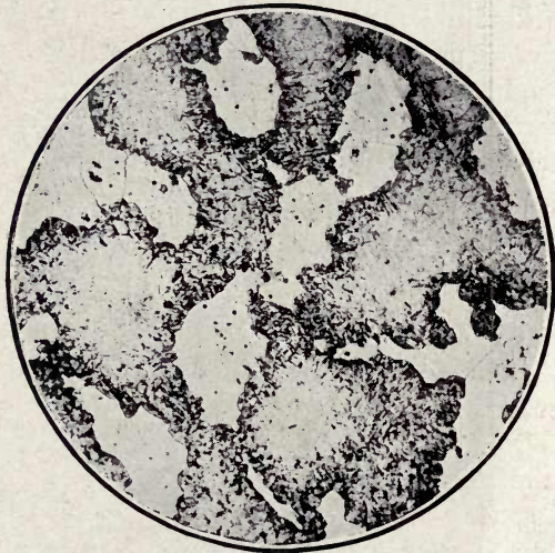
FIG. 35.—Troostite fringes within the core. \times 200 .
