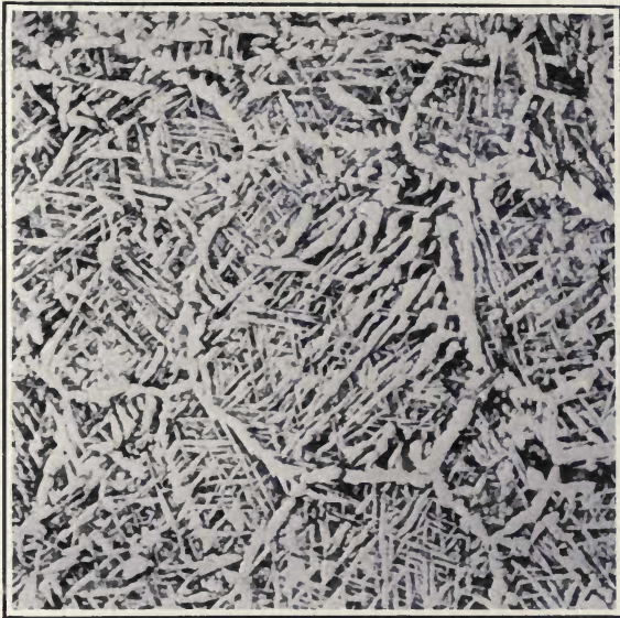
FIG. 3.—Overheated structure of mild steel. \times 25 .
