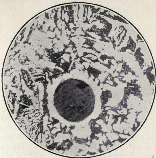
FIG. 25.—Slag globule in ferrite envelope. \times 50 .
