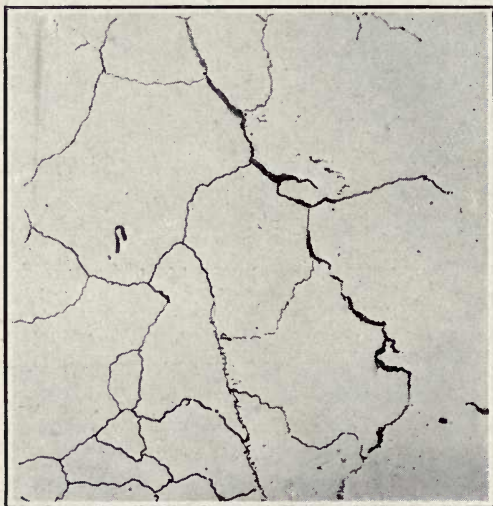
FIG. 29.—Crack proceeding along cementite outlines. \times 100 .
