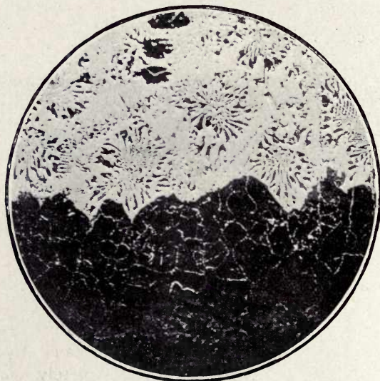
FIG. 61.—Microstructure of phosphide blister.
