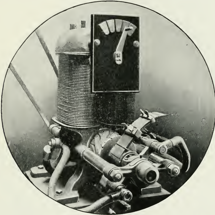
FIG. 2.—A LARGE DYNAMO USED IN THE ELECTROTYPING DEPARTMENT AT LA BELLE SAUVAGE.
