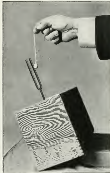
FIG. 6.—SHOWING THAT THE PRONGS OF A TUNING FORK ARE IN ACTIVE VIBRATION AFTER A BLOW.
