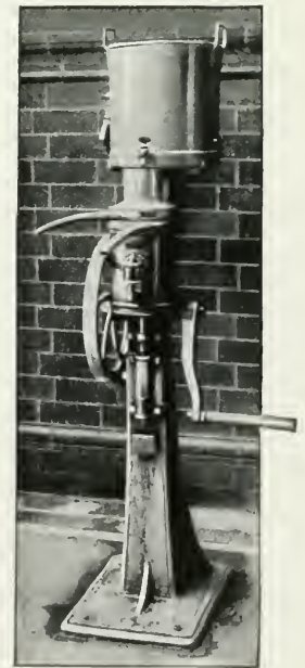
FIG. 6.—SEPARATING THE CREAM FROM THE MILK. The modern method—by means of a "separator."
