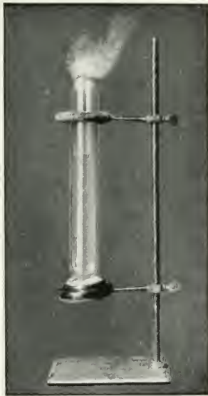
FIG. 1.—A TUBE FILLED WITH LIQUID AIR HELD IN A RETORT STAND.
