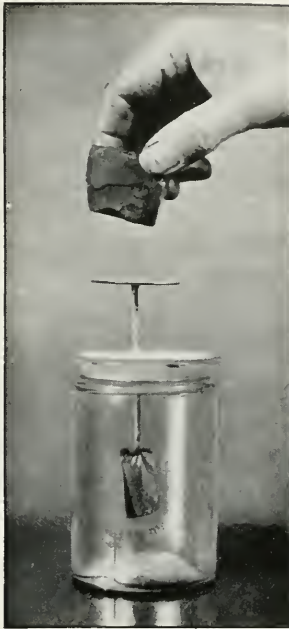
FIG. 5.—ELECTROSCOPE DISCHARGED BY THE AGENCY OF A RADIO-ACTIVE SUBSTANCE SUCH AS PITCH-BLENDE.
