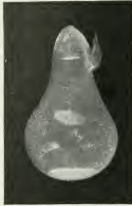
Photo: T. C. Hepworth. FIG. 2.—CROOKES TUBE, CONTAINING STRONTIUM: PHOTOGRAPHED AT NIGHT BY ITS OWN LIGHT.
