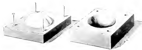
FIG. 4.—BOXWOOD MOULD FOR SUBJECTING ICE TO PRESSURE.
