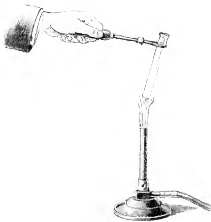
FIG. 8.—WARMING PRECIPITATE IN A TEST TUBE.
