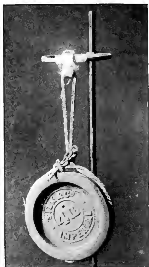
FIG. 3.—A WEIGHT SUSPENDED BY STRING AND A HOOK OF FROZEN MERCURY.
