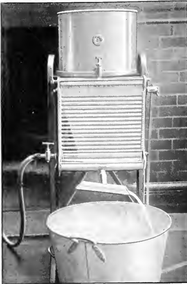
FIG. 10.—REFRIGERATOR FOR MILK AND CREAM.
