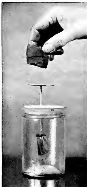
FIG. 5.—ELECTROSCOPE DISCHARGED BY THE AGENCY OF A RADIO-ACTIVE SUBSTANCE SUCH AS PITCH-BLENDE.
