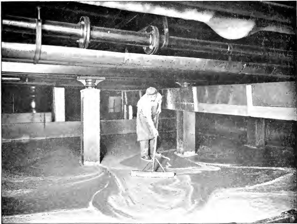
FIG. 4.—REMOVING YEAST AFTER "SKIMMING." Photographed in a brewery belonging to Messrs. Meux & Co.
