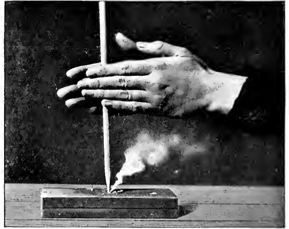
FIG. 11.—FRICTION BETWEEN HARD AND SOFT WOOD The stick is twirled rapidly between the hands.
