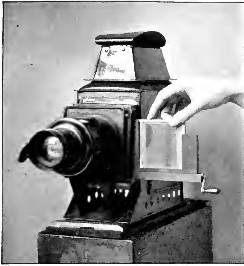
FIG. 8.—A USEFUL LANTERN: THE "SLIDE" BEING INSERTED.
