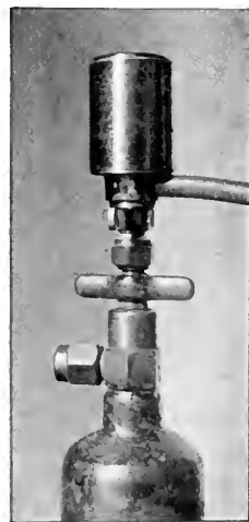
FIG. 5. — REGULATOR ATTACHED TO "GAS" CYLINDER.
