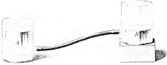
FIG. 3.—WATER FLOWING FROM A HIGHER TO A LOWER LEVEL. Note that there is a difference in "level" and a "conductor."
