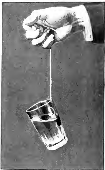
FIG. 2.—A BULLET LOWERED BY A STRING INTO THE "LIQUID" IS FROZEN FAST TO THE SIDE.
