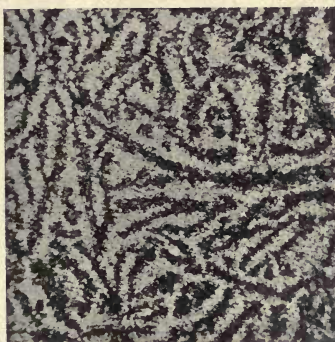
FIG. 102.—Typical structure after maximum growth has been reached. Magnified 150 diameters.
