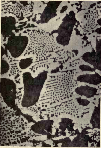
FIG. 54.—Showing process of balling-up of constituents of eutectic (sample F, 0.23 per cent. sulphur). Magnified 120 diameters.
