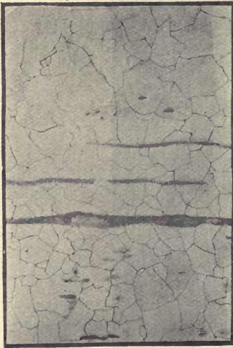
FIG. 112.—Longitudinal section of Swedish Wrought Iron as seen under the microscope. Magnified 90 diameters.
