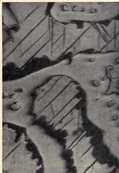
FIG. 65.—Bar 10. Magnified 1000 diameters. 6.30 per cent. Mn, 3.43 per cent. C. Rectilinear cementite needles, through solid solution. Sorbitic fringe.
