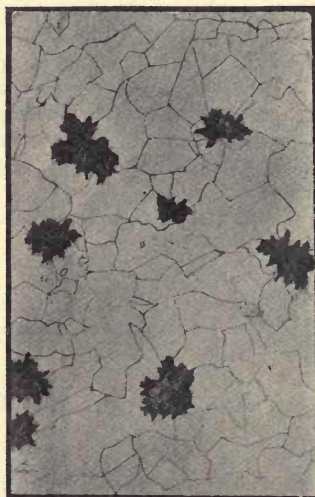
FIG. 114.—Microstructure of special Malleable Cast Iron (known in America as Blackheart). Magnified 90 diameters.
