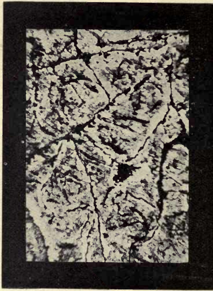
FIG. 21.—Grey cast iron. Etched \text{HNO}_3 . Magnified 52 diameters.
