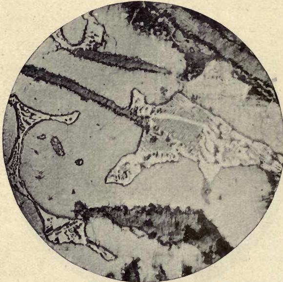
FIG. 45.—No. 3 Cargo Fleet Cleveland pig iron, showing dark sections of the graphite plates, the broken-up structure of the phosphide eutectic, and the ground mass of iron with silicon and manganese. Magnified 250 diameters.
