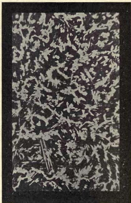
FIG. 110.—White Cast Iron. Etched. Magnified 45 diameters.
