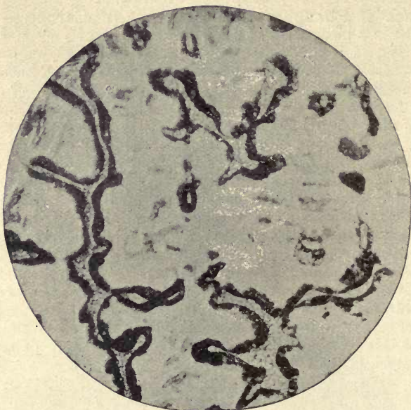
FIG. 43.—Ingot containing 1.74 per cent. phosphorus and 0.18 per cent. carbon. The mottled portions surrounded by dark borders are the eutectic of phosphide of iron. The borders are pearlite. The white ground mass is the solid solution of phosphide of iron in iron. Magnified 60 diameters.
