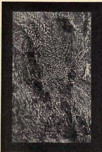
FIG. 156.—Cemented bar after heat treatment in sand. Magnified 130 diameters. Etched \text{HNO}_3 .
