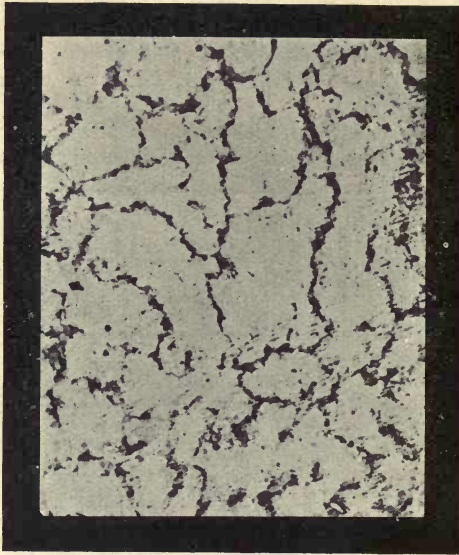
FIG. 24.—Ferro-silicon. 31.2 atom per cent. silicon = \text{Fe}_2\text{Si} .
