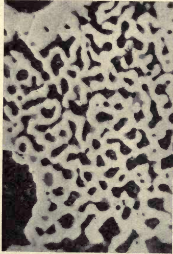
FIG. 55.—Showing eutectic area of fig. 54, highly magnified. Magnified 600 diameters.
