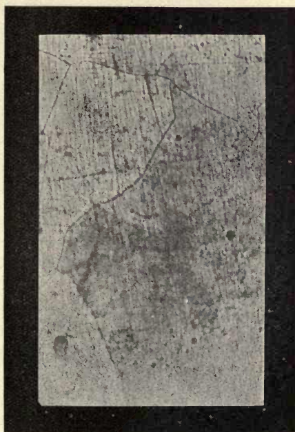
FIG. 157.—Cemented bar after heat treatment in iron ore. Magnified 130 diameters. Etched \text{HNO}_3 .
