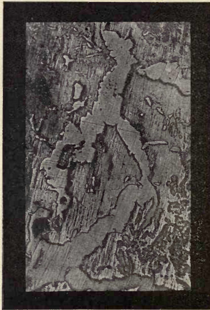
FIG. 155.—Cemented bar after heat treatment in charcoal. Magnified 130 diameters. Etched \text{HNO}_3 .
