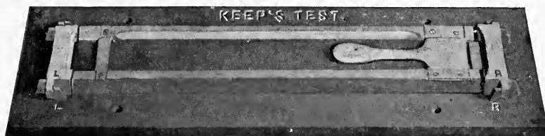
FIG. 91.—Keep's Test-bars 1" \square \times 24".
