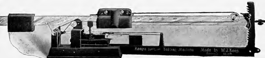
FIG. 90.—Keep's Dead-load Testing Machine, No. 10.
