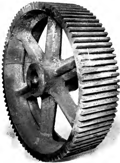
CAST STEEL PINION, WEIGHT, 4,000 LBS., REPAIRED BY THE OXY-ACETYLENE BLOWPIPE.
