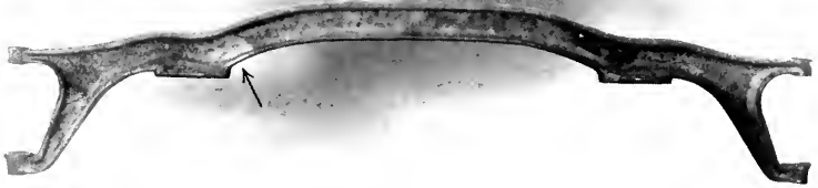
DROP FORGED AUTOMOBILE AXLE REPAIRED BY THE OXY-ACETYLENE BLOWPIPE.
