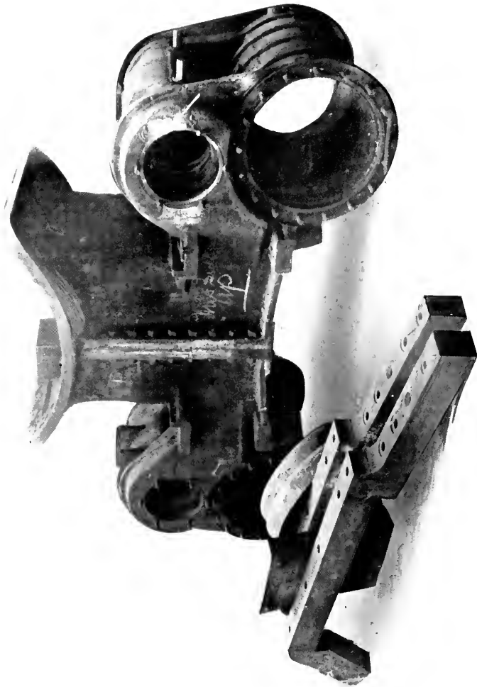
LOCOMOTIVE CYLINDER. REPAIRED BY THE OXY-ACETYLENE BLOWPIPE.
