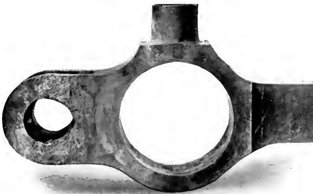
SIDE ROD OF LOCOMOTIVE REPAIRED BY THE OXY-ACETYLENE BLOWPIPE.
