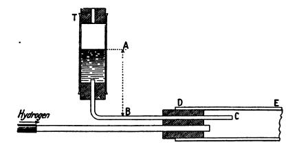
351. For most *liquids*, Sabatier and Senderens have devised an extremely simple apparatus. The liquid is conducted by a capillary tube to the interior of the reaction tube. The liquid is placed in a large vertical tube T, the lower end of which carries a stopper through which passes the vertical portion of a bent capillary tube, the horizontal portion of which passes through the stopper in the end of the reaction tube.
