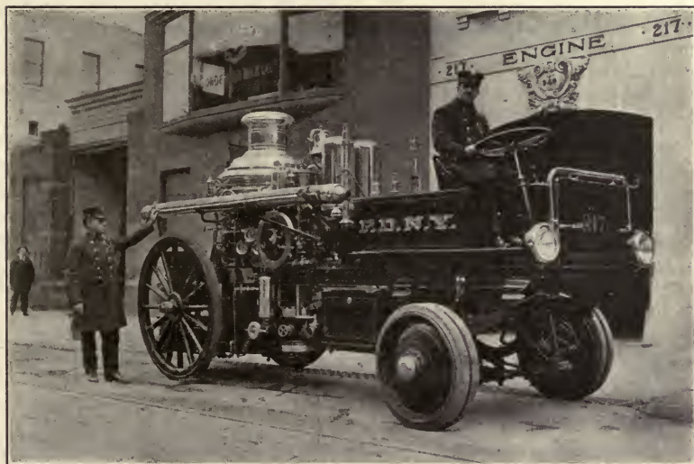
Self-Propelled Steam Fire-Engine, Period of 1917
