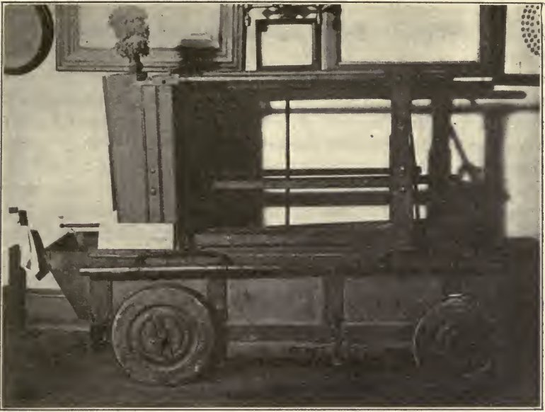
Hand-Pump Fire-Engine, Period of 1732
