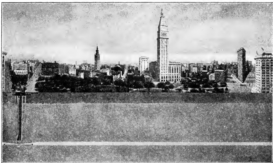
SECTION OF CITY TUNNEL OF CATSKILL AQUEDUCT WITH SHAFT UNDER WORTH MONUMENT
