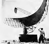
Forty-foot antenna of harbor surveillance radar.
