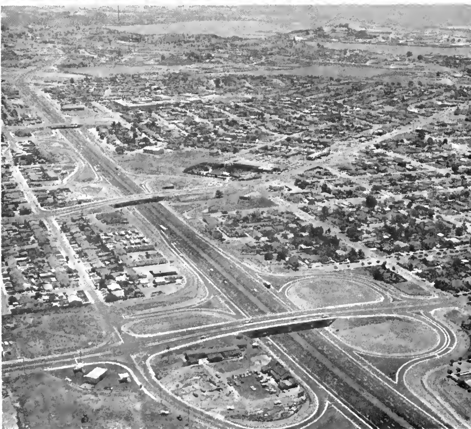
UPPER—The Moriposa Road (foreground) and Farmington Road Interchange on US 99 in Son Joaquin County, a step in the conversion of the Stockton Bypass from expressway to full freeway. LOWER—The new US 40 freeway through Vallejo. In the foreground is the Tennessee Street Interchange.
