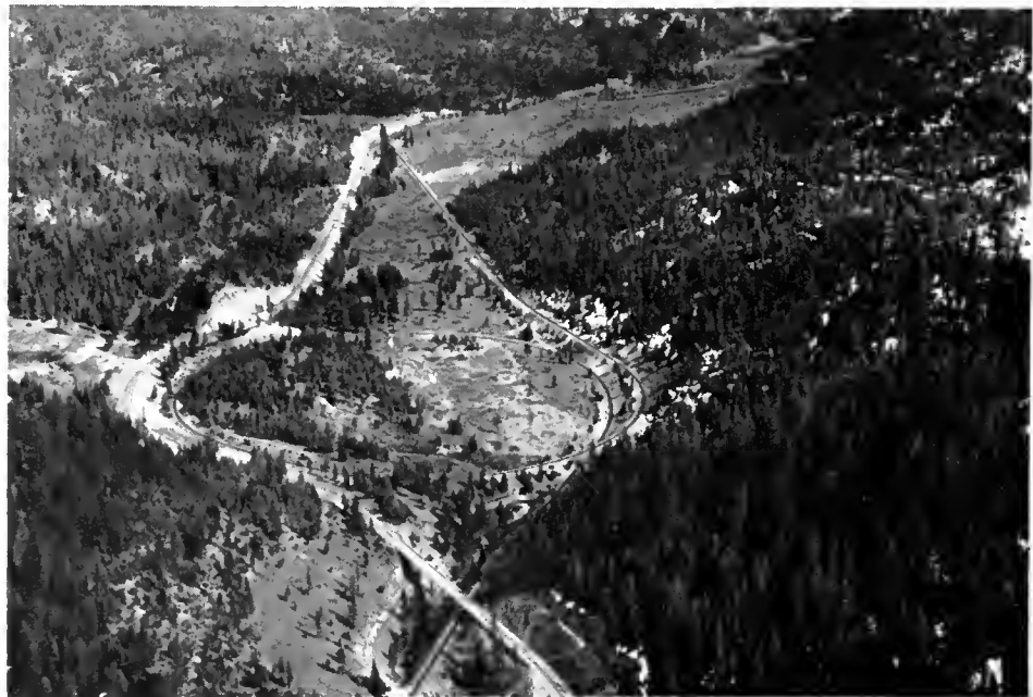
An improved section of US 40 Alternate in Plumas County a few miles west of Spring Garden. In the center is the Williams Loop on the Western Pacific Railroad Feather River Route with an overhead crossing in the foreground.
