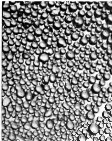
Macro-camera shows details of small objects. This picture shows typical glass "beads" used in traffic paint: Left, magnified 10 times; right, magnified 30 times.
