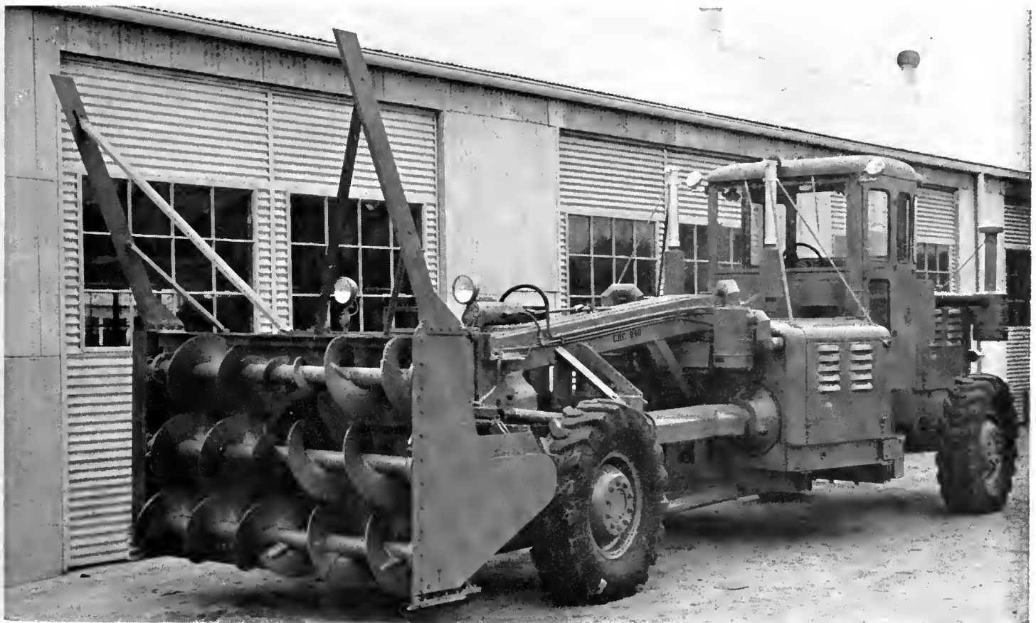
One of the auger-type rotary units mounted on a heavy-duty four-wheel-drive motor grader used by the Division of Highways in snow removal last winter
