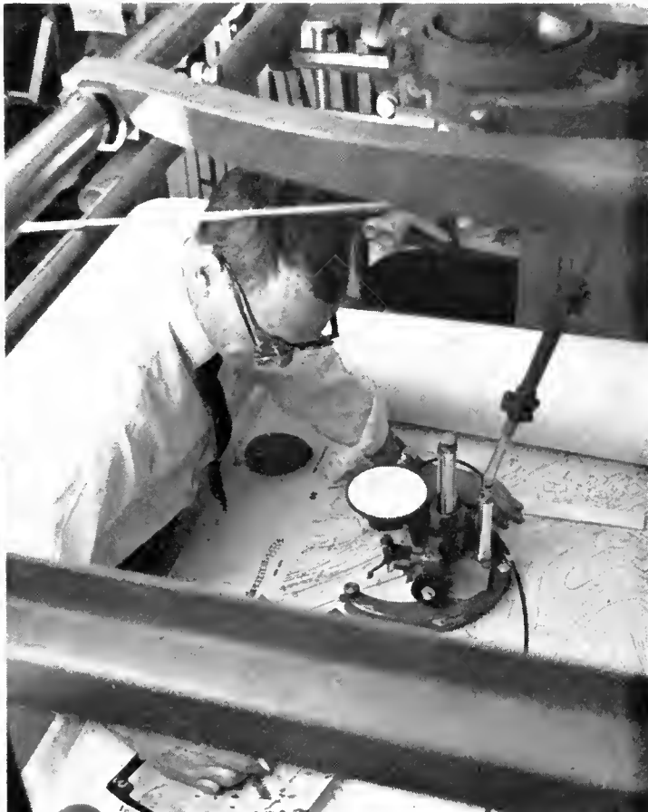
LEFT—Photogrammetrist Brennan Davis operates one version of stereo-platter, complicated mechanism for stereo-picture projection for map making. For accurate work, machine must be sturdy and built to close tolerance. RIGHT—Davis demonstrates use of stereo-platter. A three-dimensional image is projected on white disk. The operator wears special glasses, one lens red, the other blue, to get three-dimensional effect. The machine traces contours as operator allows apparent relief.
