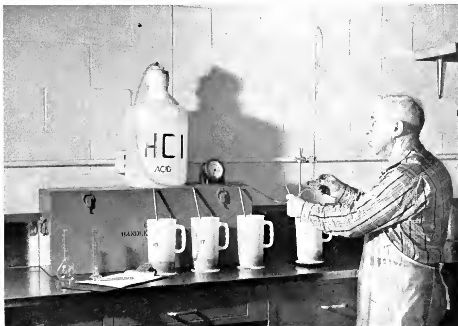
FIGURE 2—Layout for the performance of the constant neutralization procedure is illustrated above.
