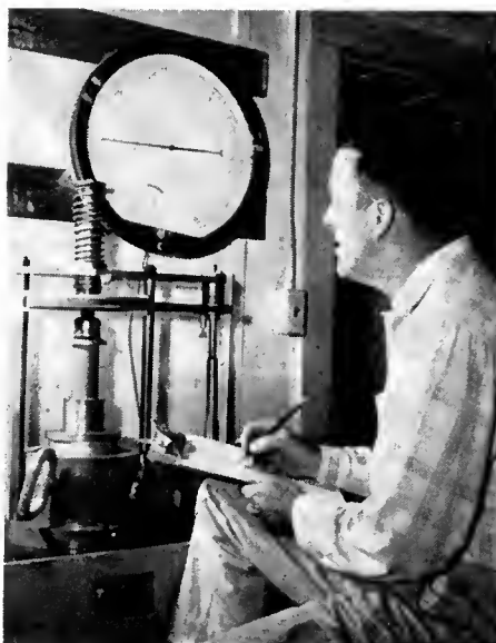
Unconfined compression apparatus for obtaining the unconfined compressive strength of clay soil
