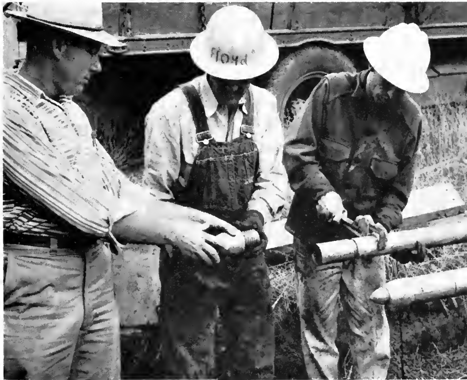
Disassembling 2-inch California sampler to remove soil samples which are contained in 4-inch-long brass tube liners
