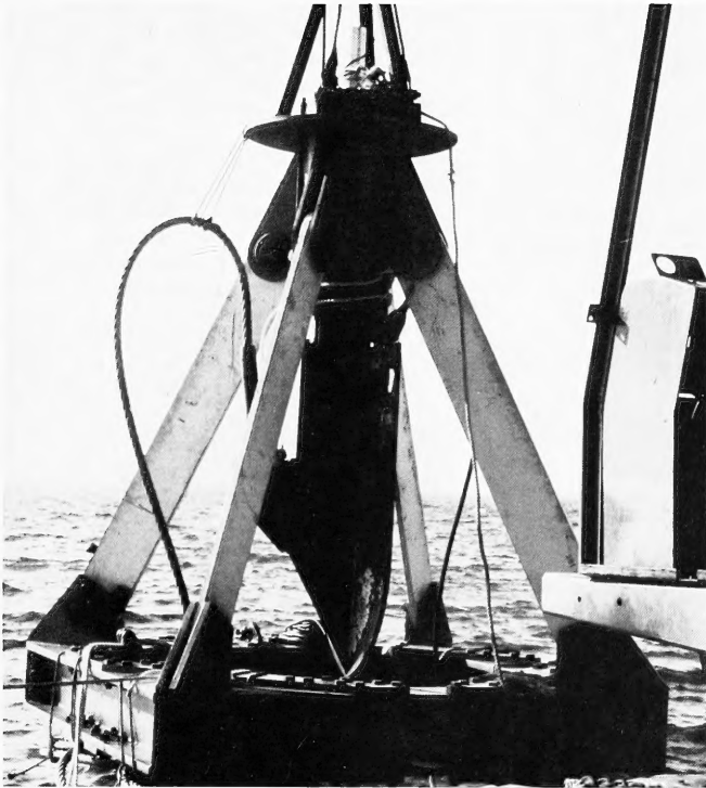
Figure 1. The CEL 100K Propellant Anchor System being deployed, loaded with a coral/sand fluke and a retrievable piston.
