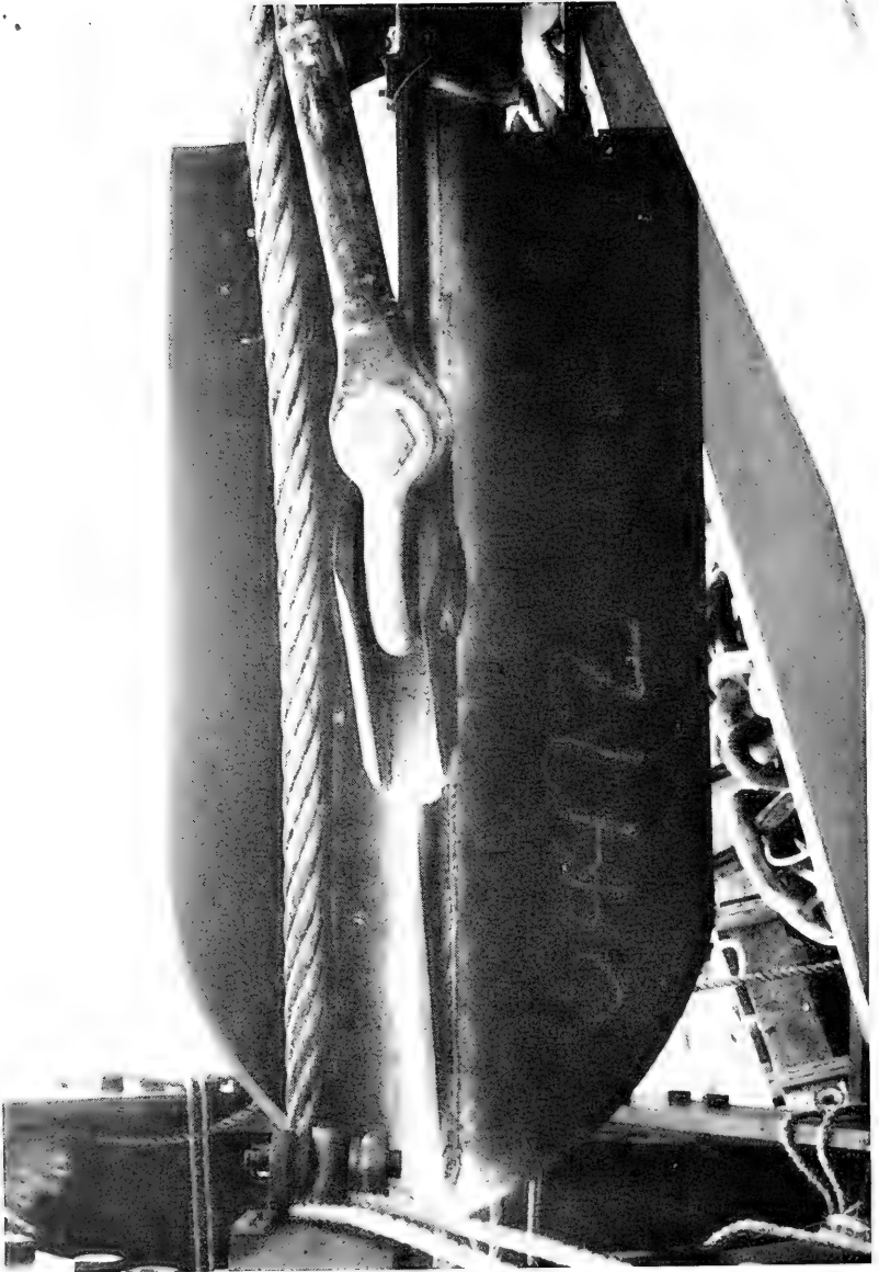
Figure 3. Projectile assembly in gun barrel with anchor load line attached.
