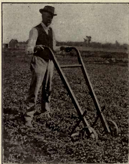
FIG. 17—DEVICE FOR CUTTING ROOTS OF CELERY PLANTS IN SEED-BED
