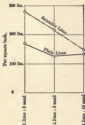
FIG. 32.—Compressive strength of plain hydraulic and selenitic limes.
