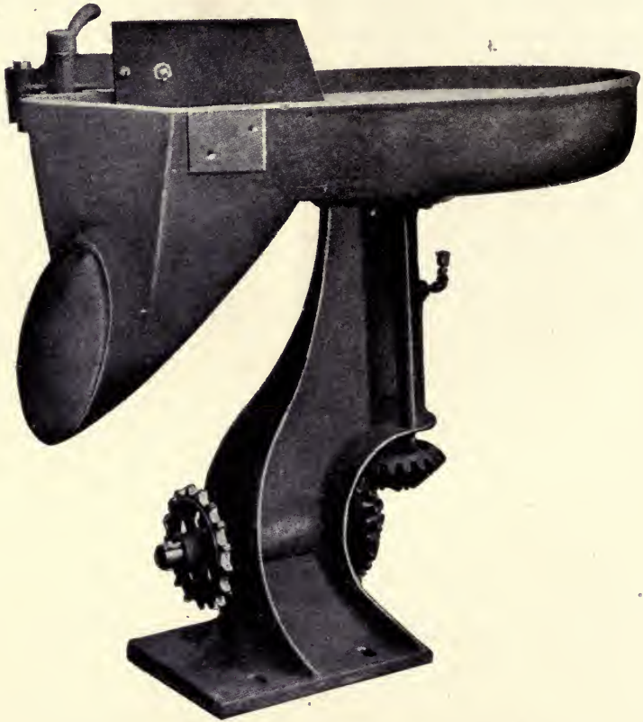
FIG. 101.—Automatic ball-mill feeder. (Smidth & Co.)
