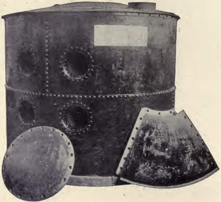
FIG. 11.—Kettle with sectional bottom. (Des Moines Mfg. Co.)
