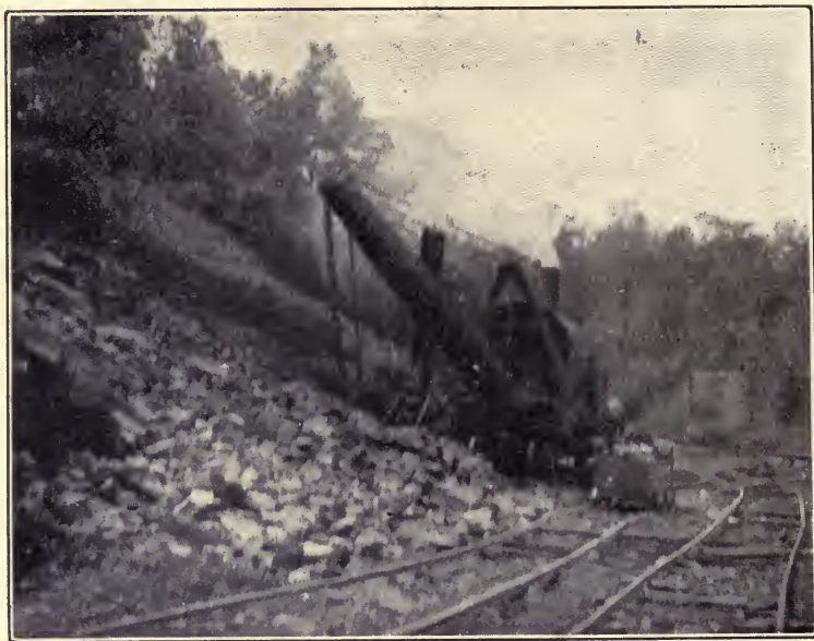
FIG. 79.—Steam-shovel handling limestone.
