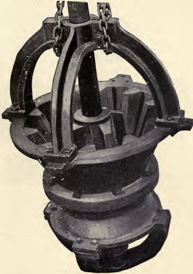
FIG. 6.—Cracker for intermediate reduction. (Butterworth & Lowe.)
