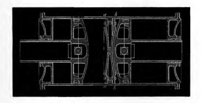
"With regard to the supposed rapid transmission of heat through the 'iron partition of the two cylinders,' you will find on referring to the section that no transmission of heat can take place, since the two bottoms are separated by a stationary body of air or vapor. In the ordinary cylinderbottom, the outside of the metal acquires, during regular working of the engine, a permanent temperature, attended by a constant loss of heat radiated into, and continually ab-
