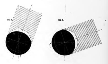
of the sun during the observation influences the accuracy of the indication. This will be readily comprehended. Fig. 2 represents the bulb of a thermometer exposed to the rays when the sun's zenith distance is 65 deg.; Fig. 3 representing the bulb when the zenith distance is 18 deg. 23 min., the latter being the minimum at the observatory of the Roman College, where the thermoheliometer described in Chapter XV. has been long employed for the purpose of ascertaining
