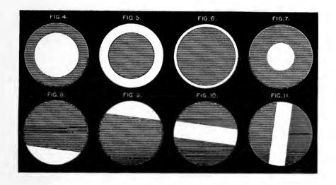
our attention. Fig. 6 represents the solar disc covered by a circular screen 145.25 millimetres in diameter, excluding the rays excepting from a narrow zone, the mean width of which is situated 49" from the border of the photosphere. Fig. 7 shows a screen excluding the solar rays excepting from the central portion, the area of which is precisely equal to the area of the narrow zone in Fig. 6. The following table shows the intensities transmitted to the actinometers
