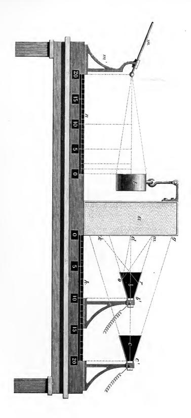
APPARATUS FOR MEASURING RADIANT HEAT. DESIGNED BY JOHN ERICSSON. CONSTRUCTED AT NEW YORK, 1873.
