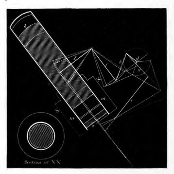
perceived on inspection that the upper end of the cylinder will be subjected to a concentration of heat many times greater than the concentration at the lower end. Referring to the accompanying diagram representing a vertical section of the machine, it will be seen that the working-cylinder, open at the lower end, contains two pistons, a working-piston a and an exchange-piston b. The working-piston is
