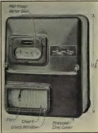
FIG. 32.—The Westinghouse Type RA demand watt-hour meter.
