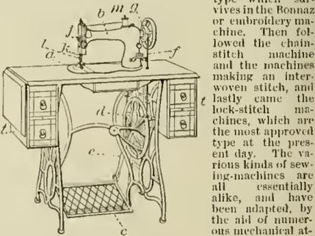
almost every kind of sewing that can be done by hand. In figs. 1 and 2 (Singer sewing-machine) a is the frame and cloth-plate or bed-plate; b, arm; c, machine; d, pitman; e, main driving-wheel; f, band; g, small driving wheel at
