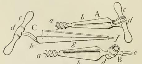
A, B, tap-borers with auger-bits *a*, and taper reaming cutters *b*. A and C have auger-handle at *c* socketed at *d*; B, besides the socket for the auger-handle at *c*, has a shank *e* for the use of a bit-stock; C has a gimlet point at *f*, and a hollow half-cone cutter *g*, with sharp beveled edges at *h*.
