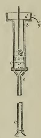
Suction-pump. a, piston; b, barrel; c, suction-pipe; d, pump-back or pump-box; e, valve in piston; f, valve which admits water into the barrel; g, spout, pump-dale, or date.
