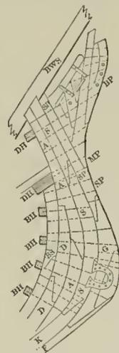
Stem and allied parts. S, stem; K, keel; A, apron; D, deadwood; SS, sternson; DH, deck-hooks; BH, breast-hooks; SP, stem-piece, or independent piece; MP, main piece, or lace-piece; BP, bobstay-piece; WS, bowsprit; G, girce; F, false keel. (The dotted lines show bolts.)
