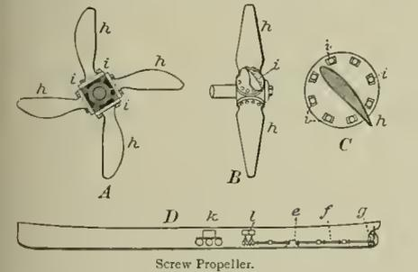
Screw Propeller. A, sectional elevation, the section being through shaft and hub, showing method of attaching blades h by bolts i, j, k, l, m, n, o, p, q, r, s, t, u, v, w, x, y, z; B, side elevation; C, cross-section of blade, on larger scale; D, diagrammatic view of hull of a screw-propeller ship, in which k shows position of boiler; l, the engines; f, propeller-shaft; e, thrust-block; g, propeller.
