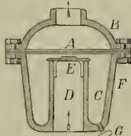
Sand-trap (in section). F, cast-iron body; E, cover; A, finely perforated diaphragm; D, induction-port for water; E, valve. (Water enters through D, and the sand is collected in C.) G, plug for clearing out sand.
