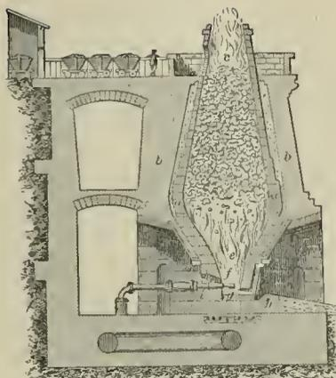
Smelting-furnace. a, fire-brick lining; b, masonry; c, opening in the side of the upper part of the furnace through which it is charged; d, hearth or crucible; e, shaft; f, throat; g, dam-stone; h, twyer. That part lying below the widest diameter, above the boshes, is called the shaft.
