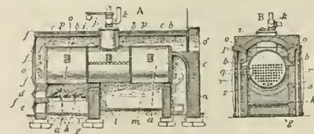
Horizontal Cylindrical Tubular Steam-boiler.
