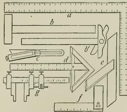
*a*, carpenter's square (of iron or steel); *b*, *b'*, draftsman's T-squares of wood; *b'* having a head adjustable at any angle; *c*, bevel-square, the blade of which can be set either square or at any angle; *d*, center-square; *e*, miter-square; *f*, carpenter's try-square; *g*, square with adjustable beads and with vernier scale for measuring diameters, also called vernier calipers.
