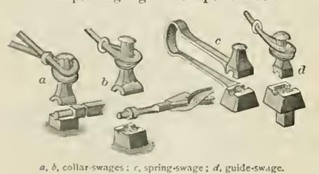
a, b, collar-swages; c, spring-swage; d, guide-swage.
