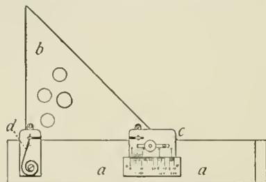
*a*, straight-edge; *b*, triangle moving on *a* for a distance determined by the set of the micrometer-scale; *c*, spring for releasing triangle and keeping it in the end of its slot.
