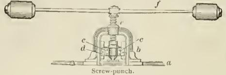
a, bed; b, yoke, on the inner sides of which are slides for the cross-head c; d, the punch proper; e, nut for the screw f, weighted lever by which the screw is made to exert its power upon the punch d.
