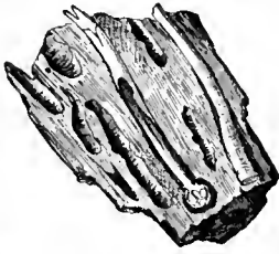
Piece of Wood Perforated by Teredos.
